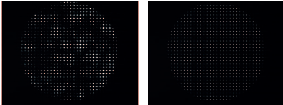
Figure C.5: The spot diagram of the plane wavefront of the model eye when the diffuser is still (left) and when it is rotated by the motor(right).
