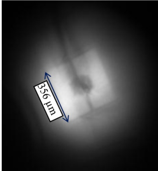
Fig. 4.2: Emitter size on the CCD corresponding to 121 \mu m on the retina.
