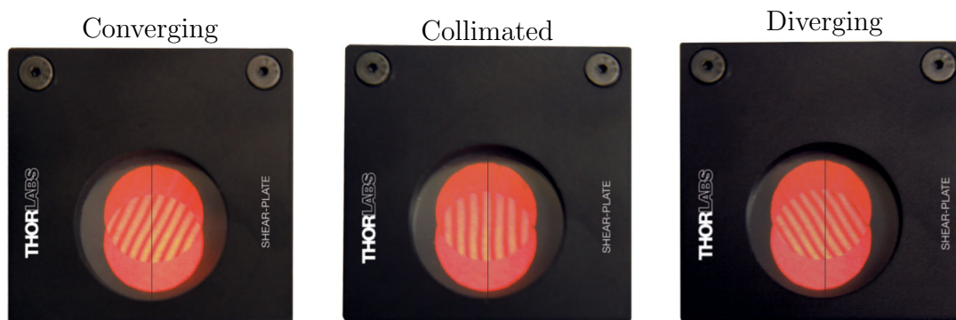
Fig. 6.1: The shear plate uses two reflections of the same beam, separated by an optical path difference. Their interference causes a pattern that defines the beam’s divergence. [108]
