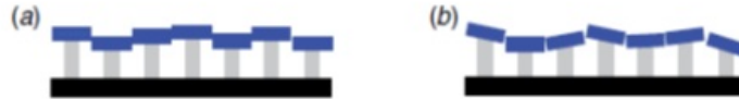
Fig. 2.1: Segmented deformable mirrors: (a) piston only and (b) piston, tip and tilt. [20]
