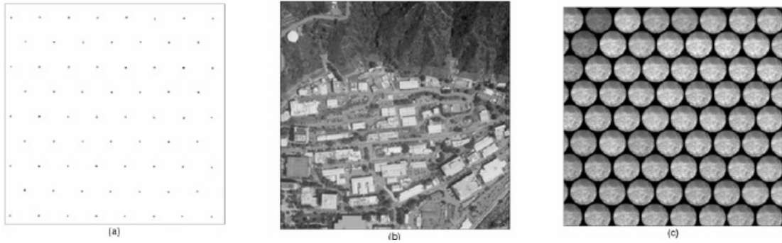
Fig. 3.15: (a) A point source spot-image of a Shack-Hartmann sensor. (b) An example of an object scene image used to create an SH extended-scene image. (c) The SH extended-scene created by convolving (a) with (b). [84]
