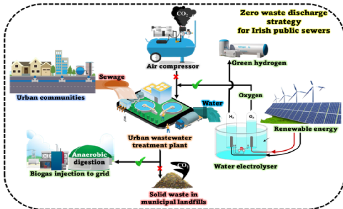
Fig. 2. Proposed waste treatment scheme to convert Irish wastewater treatment plant to green infrastructure. In this new scheme, wastewater plants will replace conventional methods of pumping air through a compressor with pumping oxygen from water electrolysis and using renewable energy. Regular landfilling of treatment plant sludge is replaced by using sludge as feedstock for anaerobic digestion.
