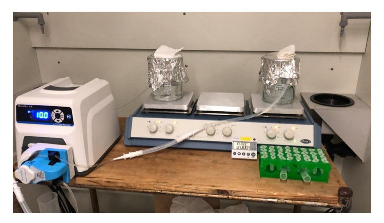
The laboratory scale silicone membrane contactor system consisting of two beakers with the first beaker (feed) having solution rich in VFAs/alcohols connected to the second beaker (draw) with de-ionised (DI) water that is temperature controlled and stirred using a magnetic stirrer, inside which the silicone membrane is immersed for extraction tests.
