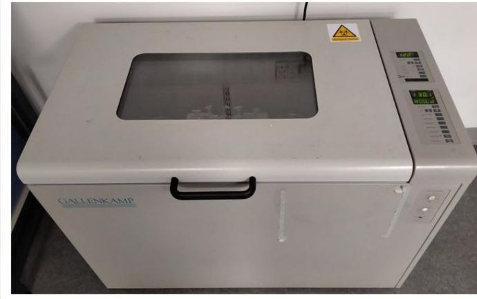
Toxicity test for investigation of the effect of concentration of selenate and selenite on anaerobic digestion utilising DAF slurry is conducted in 60 ml working volume (30 ml DAF slurry and 30 ml distilled water) incubated at 30 °C on an orbital incubator shaker (*Gallenkamp*) at 120 rpm. 1.5 g of wet anaerobic sludge is used as inoculum for the study.
