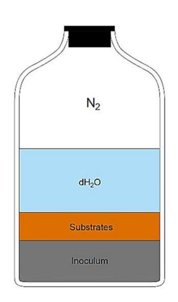
Working Volume  $\rightarrow$  150 mL Head Space Volume  $\rightarrow$  100 mL Mesophilic AD  $\rightarrow$  37 °C Wet AD  $\rightarrow$  1.8% TS Inoculum/Substrate  $\rightarrow$  1.5 VS/VS
