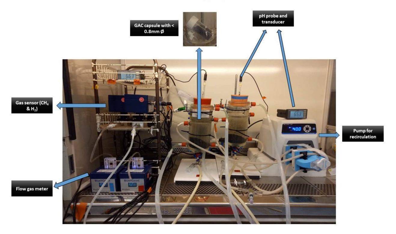
This set-up is a fed-batch reactor with side stream recirculation flow at 1.5 m/h and 37°C. It is fed with real dairy wastewater taken and with gas sensors ( $CH_4$  and  $CO_2$ ) and flow meter attached at the end. One reactor is taken as the control while GAC is added to the other, contained in a small capsule with < 0.8 mm diameter holes.
