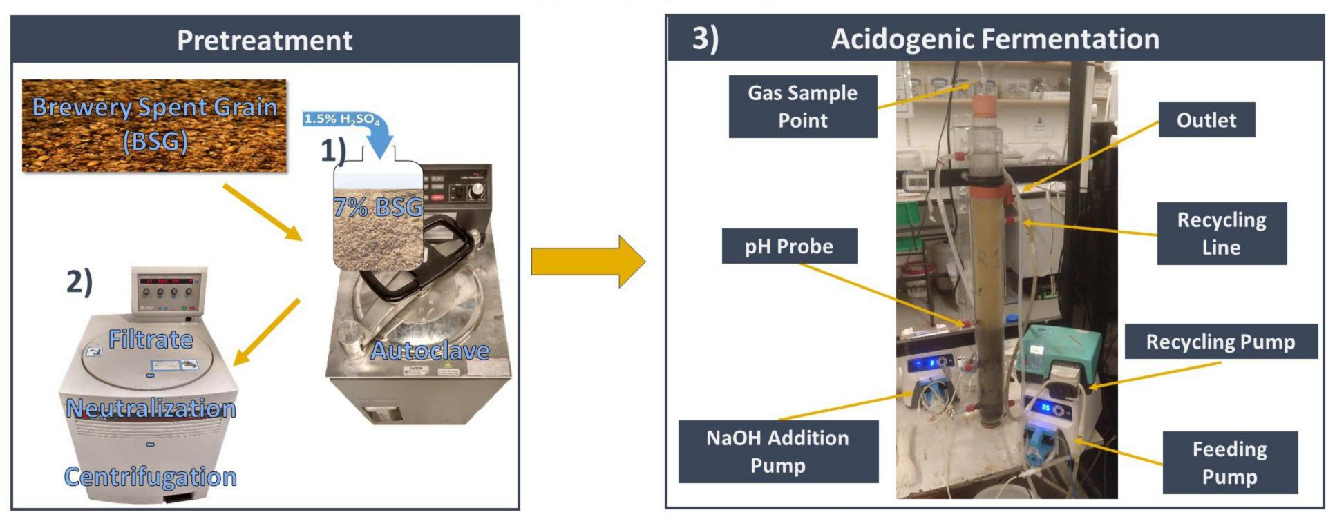
This process is divided mainly in three different steps. The first two steps are related with the pretreatment process, 1) hydrolysis and 2) recovery and neutralization, of the brewery spent grain to obtain a leachate rich in carbohydrates easily fermentable by microorganism. The third step is the acidogenic fermentation. The leachate is fed under different hydraulic retention times in the reactor. Temperature, pH and up-flow velocity are kept constant.
