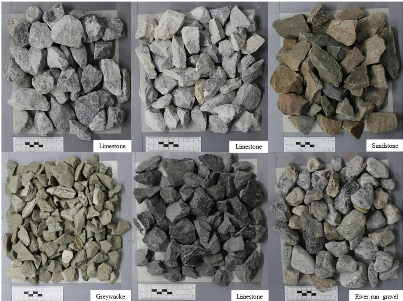
**Figure 3.** A selection of Q50 mm aggregates of different lithologies.
