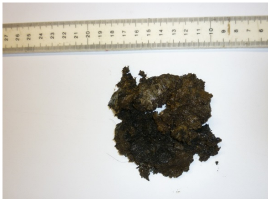
Lime stabilised biosolids
