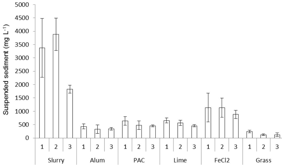
815 Fig 5 Average flow weighted mean concentrations of suspended sediment in runoff.
