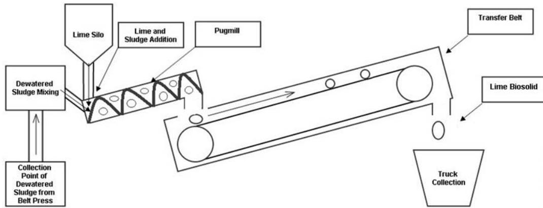
**Figure 4.7.** Illustration of a standard mixing apparatus at a WWTP
