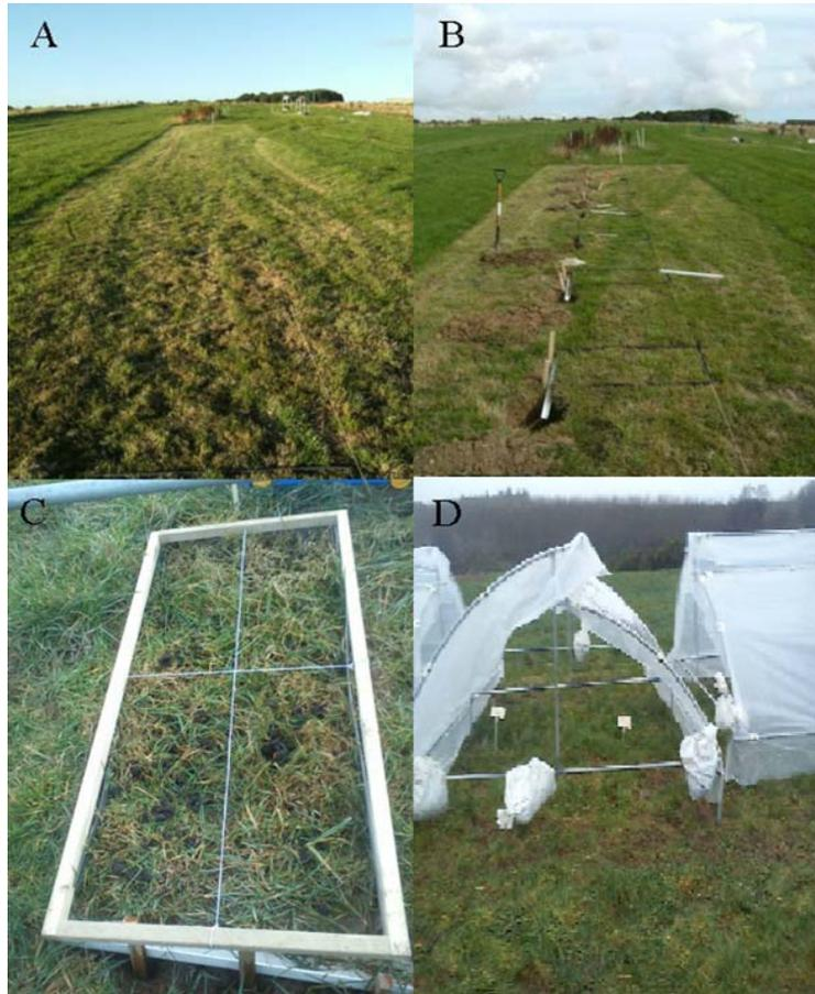
**Figure 5.4.** A) and B) show site set up, C) Quadrant used to apply biosolids evenly, D) Rainout shelters to excluded natural rainfall
