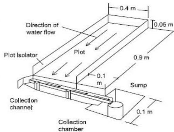
**Figure 5.2.** Picture of micro-plot fitted with runoff off collection channel and micro-plot set up.
