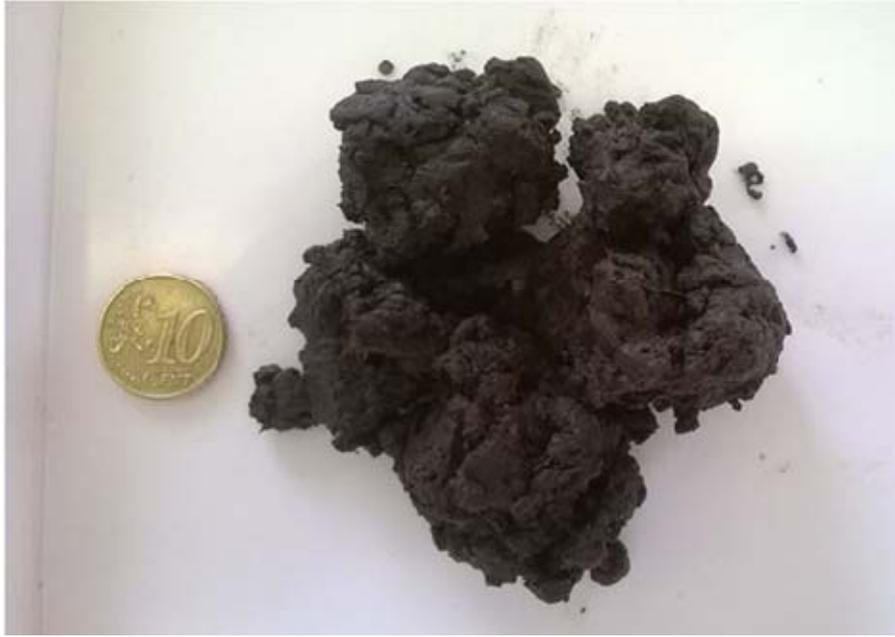
**Figure 2.3.** A 50 g sample of anaerobically digested biosolids (ADIRE)
