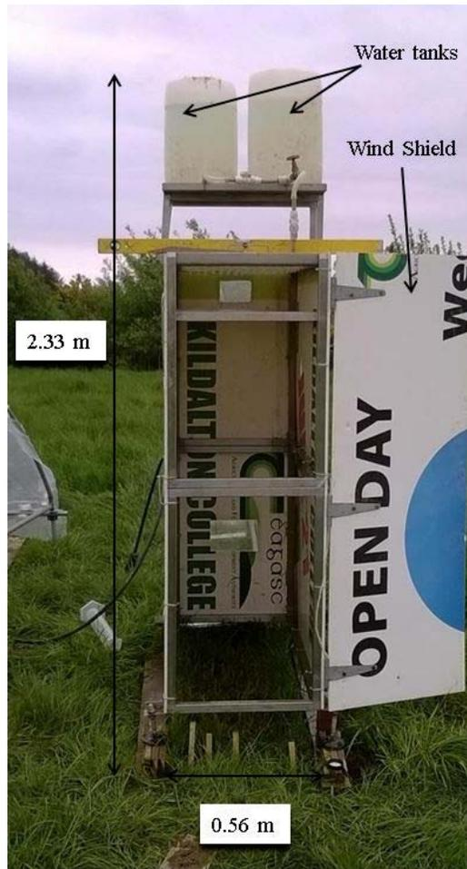
**Figure 3.2.** Amsterdam-styled drip-type rainfall simulators fitted with wind shield in use in field.
