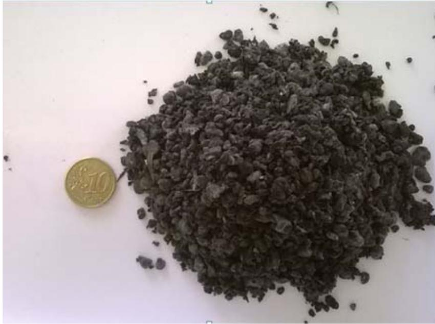
**Figure 2.4.** A 50 g sample of thermally dried biosolids (TD)
