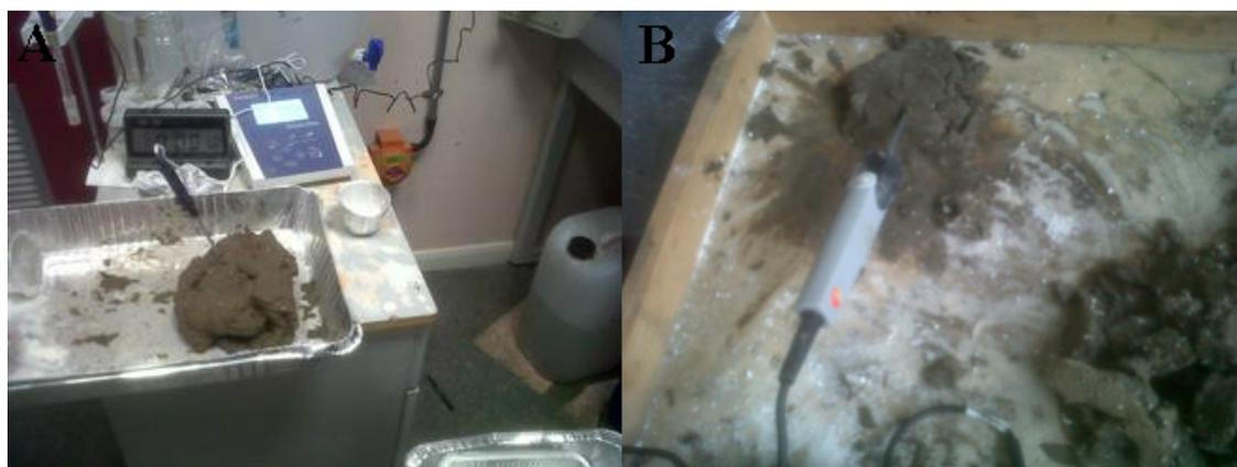
**Figure 4.2.** The experimental setup for the preliminary test. A) – temperature monitoring of 2 kg sludge cake and B) – a temperature probe close up.
