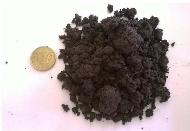
**Figure 5.3.** Anaerobically digested biosolid source from END-O-SLUDGE, 2014 (ADUK)
