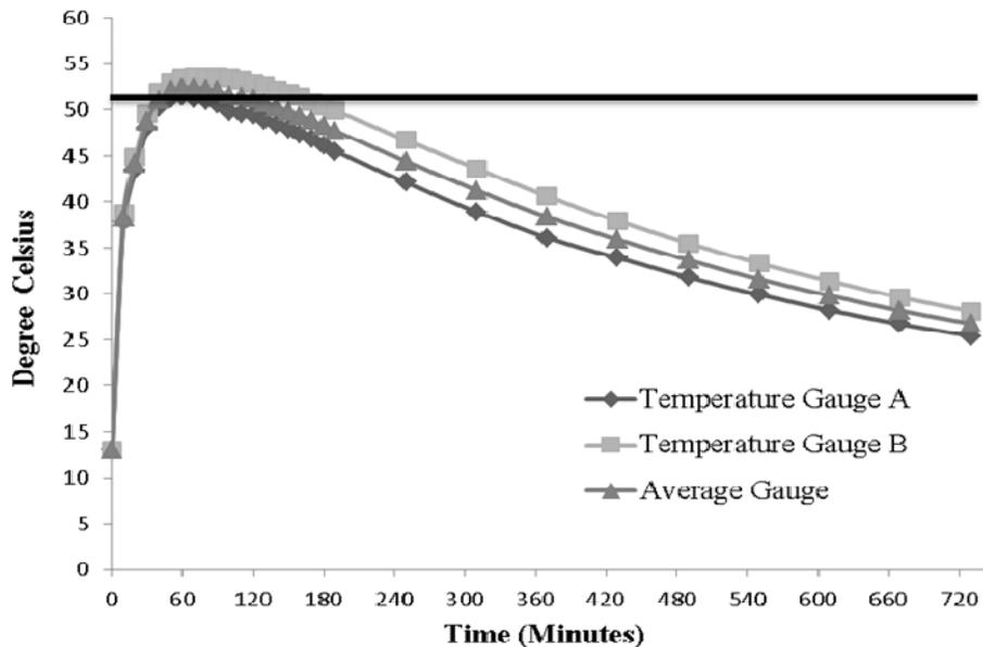
**Figure 4.5.** Temperature vs. time over 12 hr. Horizontal bar indicates 52°C, which is the temperature guideline (Fehily, Timoney and Company, 1999)
