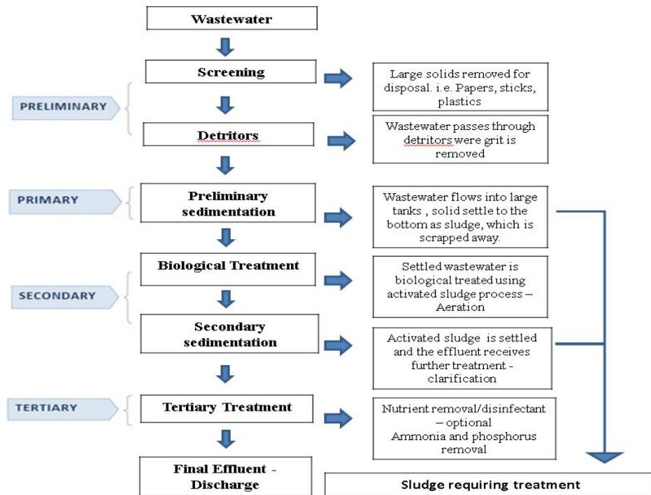
**Figure 2.2.** Illustration of a simplified wastewater treatment process (adapted from Antille et al., 2011; Metcalf et al., 2003).
