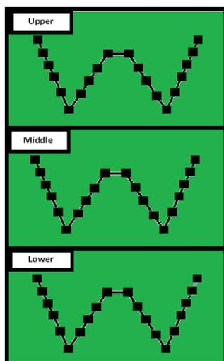
**Figure 5.1.** The “W” soil sample procedure outlined in the S.I. No 610 2010. This soil sample procedure was carried out for the Upper, Middle and Lower sections of the field
