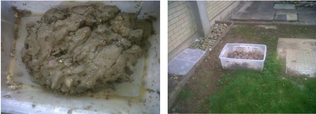
**Figure 4.4.** Shows final lime-sludge mixture and storage outside for 48 hours
