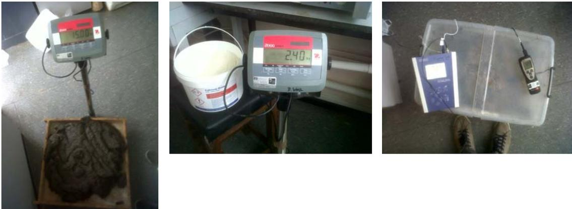
**Figure 4.3.** The measurement of lime and sludge, and sealed container mixture with temperature probes inserted.
