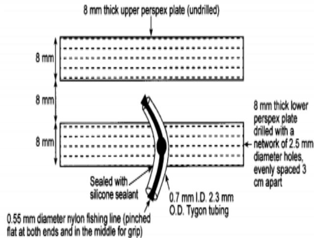
**Figure 3.1.** Principal components of the rainfall simulator (top) and of Perspex plate (bottom)
