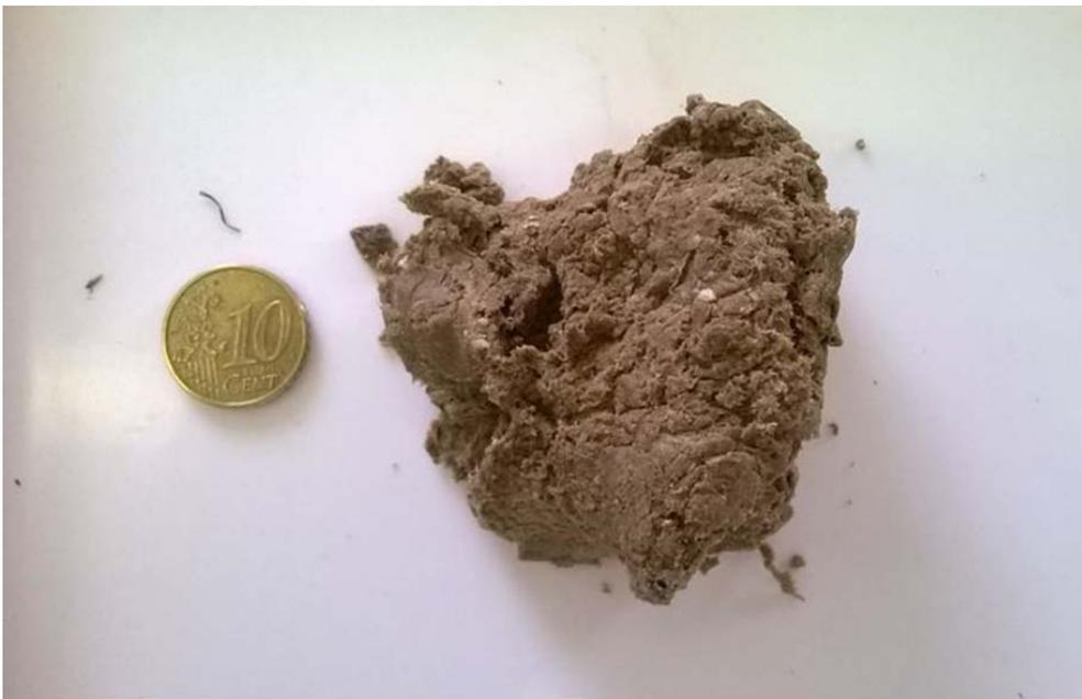
Figure 2.5. A 50 g sample of lime stabilised biosolids (LS).
