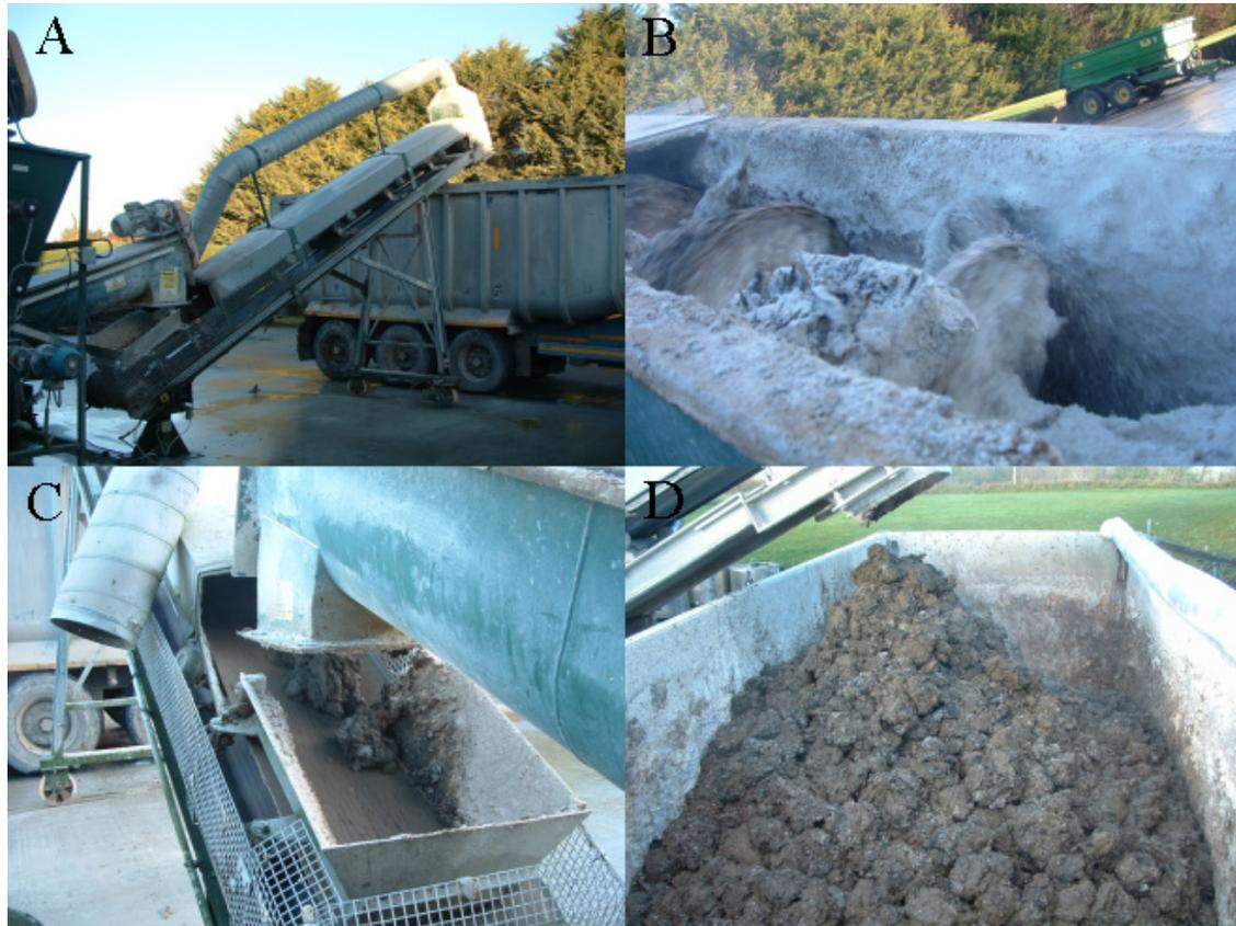
**Figure 4.6.** A) Standard lime-sludge mixing apparatus at a WWTP, B) Pugmill Augers, C) completion of sludge and lime mixture on transfer belt, D) truck collection.
