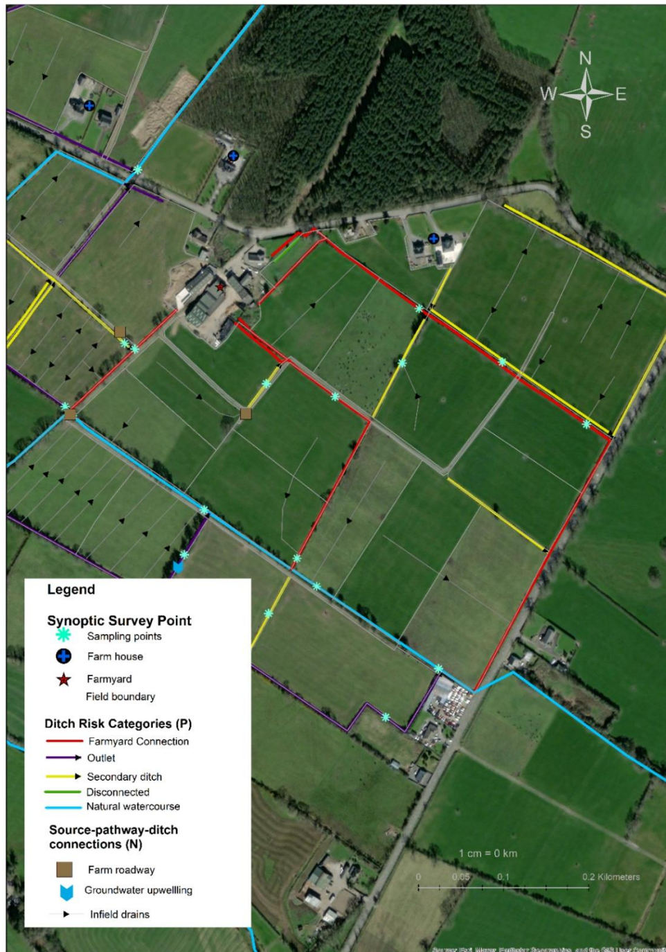
Figure 3.2 Example of a farm output map (for Farm 5) showing the ranked classification risk along the open ditch network for P (colour coded into categories of connectivity risk) and all conceptualised N open ditch connectivity pathways to individual open ditch sections. For in-field drains, arrows indicate fall and flow direction towards open ditch sections, with a particular P risk indicated by the existing colour coding scheme of Moloney et al. (2020).
