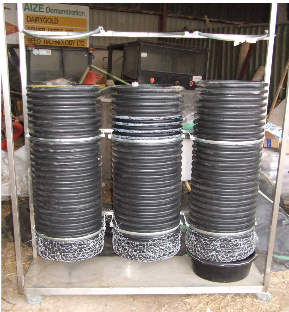
Figure 5.3 Sand filters as constructed – three replicate
