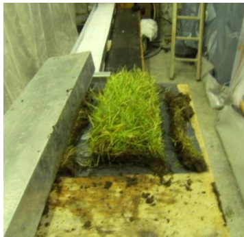
Soil sample trimmed immediately prior to placement
