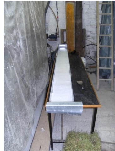
Runoff box ready for soil to be placed
