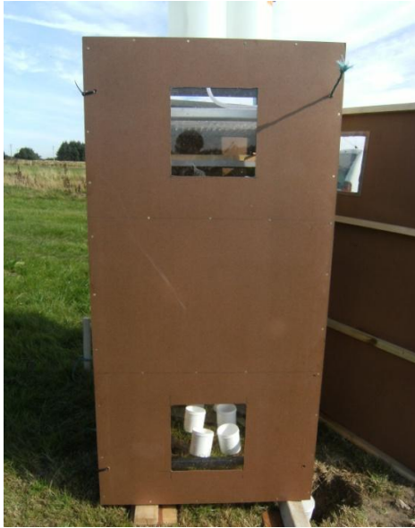
Wind shield used to prevent rain from blowing rain
