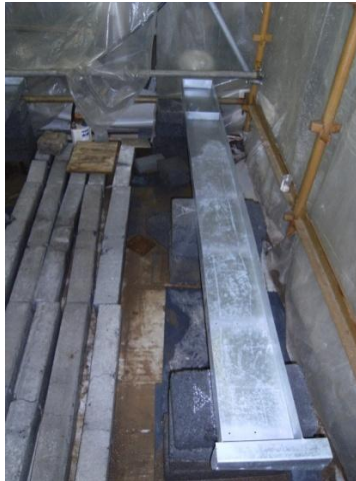
Runoff box cleaned prior to each rainfall simulation
