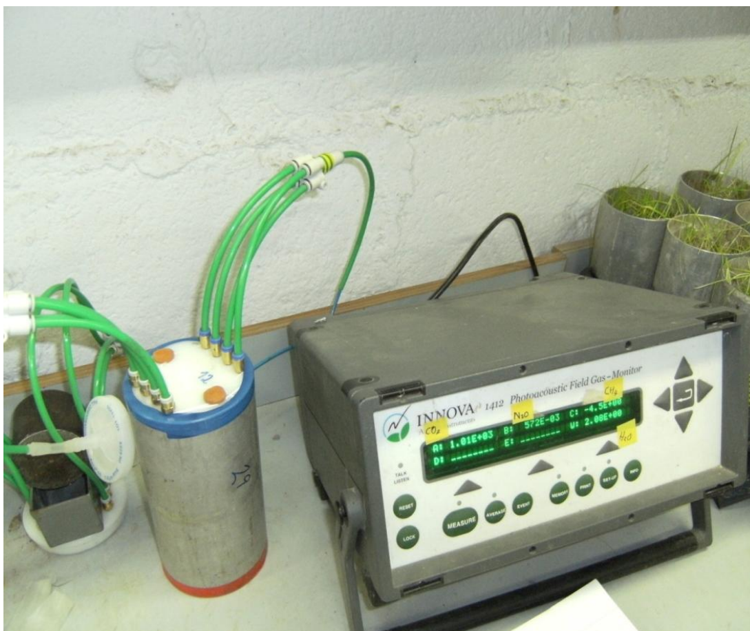
Figure 5.4 Photograph of PAA during carbon dioxide, methane and nitrous oxide measuring period
