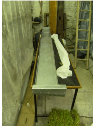
Muslin cloth cut to length to prevent soil loss and aid drainage
