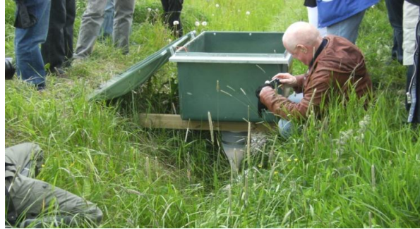
Figure 2.11 Schematic and photo of ferric-sulphate doser in operation in Jokioinen, Finland (Narvanen et al., 2008)
