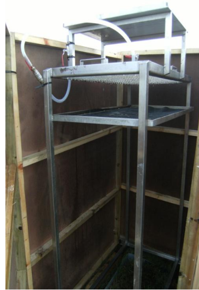
View of rainfall simulator before rainfall starts
