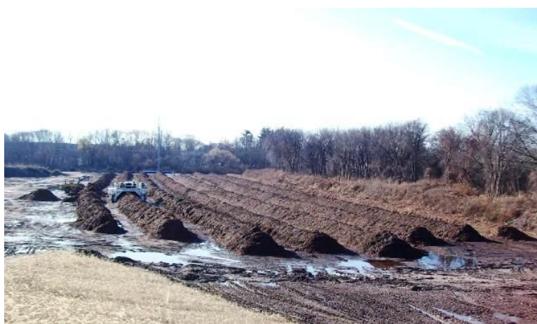
Figure 1.12 Windrow composting system (source windrow systems ) (accessed Feb. 2017).
