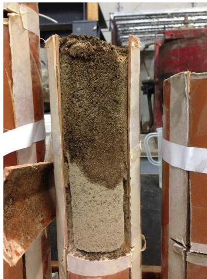
Figure 2.7 Evidence of clogging in a sand filter.
