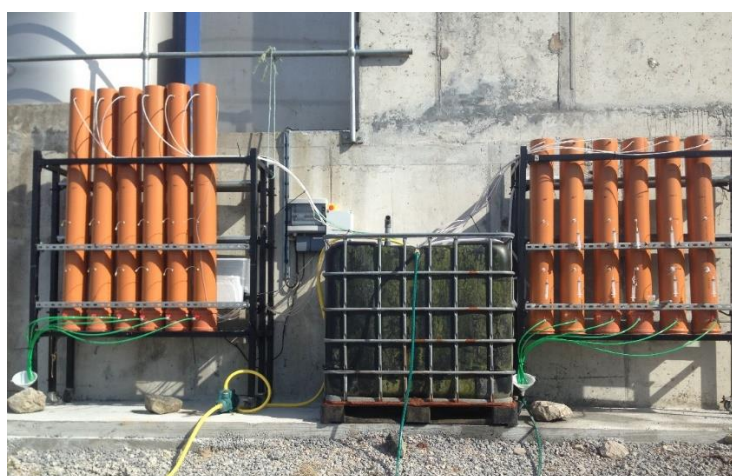
Figure 5.2 Six continuous and six intermittently loaded columns in place at the pilot-scale study location.
