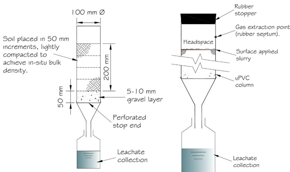
Fig. 1. Schematic diagrams of (A) typical column setup for leachate sampling and (B) column setup during gas sampling (Not to scale).
