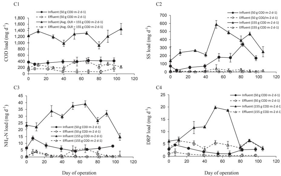
**Fig. 5.** Impact of organic loading rates on COD, SS,  $\text{NH}_4\text{-N}$  and DRP mass removals. The filter material used was 10–20 mm Sitka spruce woodchip, 1 m deep. Error bars indicate standard deviations.
