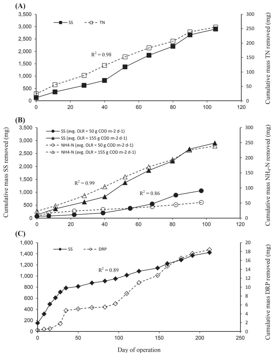
**Fig. 4.** Correlations between cumulative mass removals of suspended solids (SS) for 1 m deep  $\times$  0.1 m  $\varnothing$  woodchip filters ( $n = 3$ , each set) and (A) TN loaded at 120 g COD m<sup>-2</sup> d<sup>-1</sup> (B)  $\text{NH}_4\text{-N}$  loaded at 50 and 155 g COD m<sup>-2</sup> d<sup>-1</sup> respectively and (C) DRP loaded at 35 g COD m<sup>-2</sup> d<sup>-1</sup>. Correlation coefficients, ( $R^2$ ) indicated.
