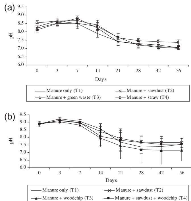
Fig. 3. Compost pH for Trial 1 (a) and Trial 2 (b).
