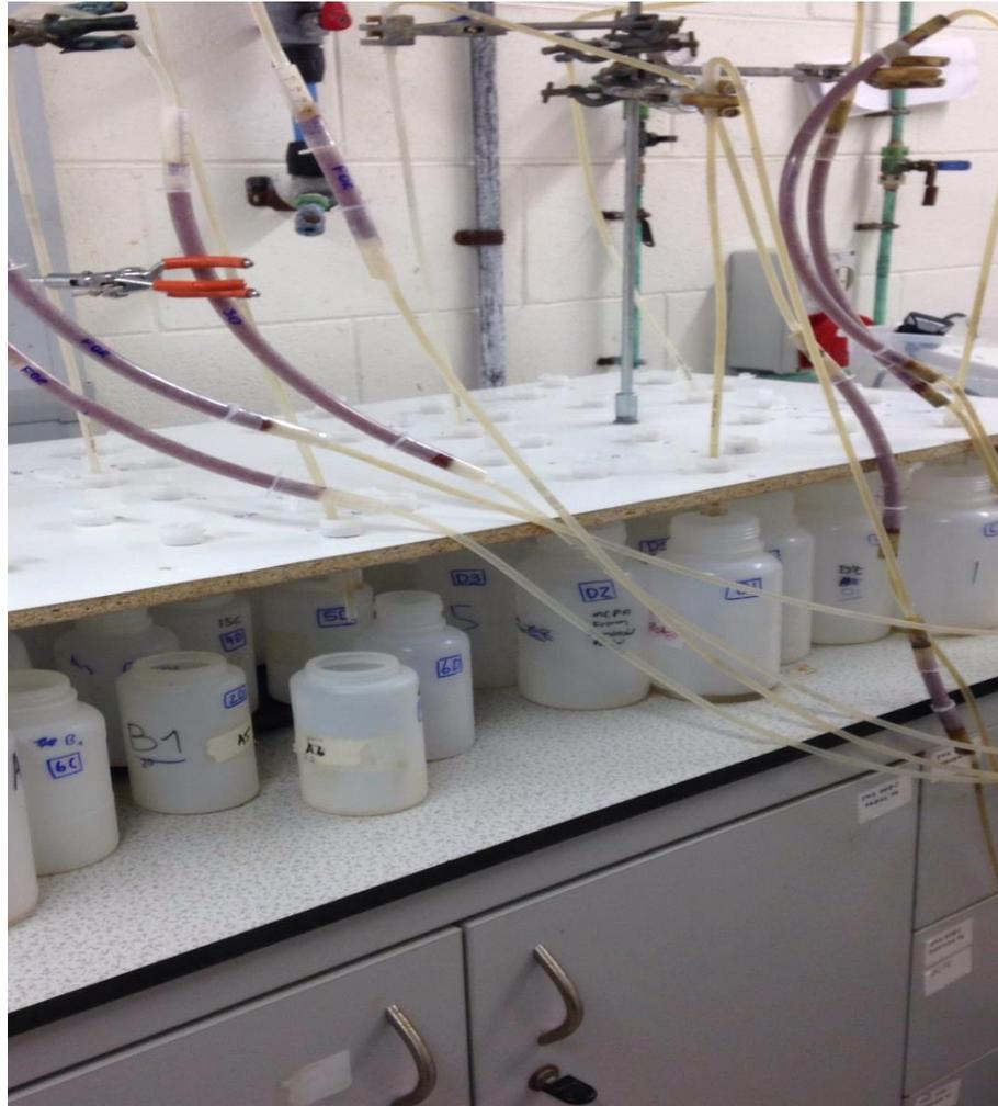
**Figure 5.1** Image of the rapid small-scale column tests (RSSCT) set-up used in this study.
