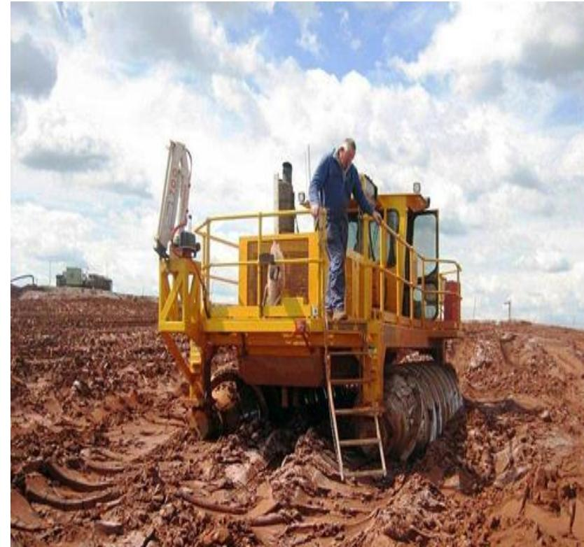
**Figure 2.2 (a)** Schematic of a BRDA, which incorporates the dry stacking or TTD technique for storage of bauxite residue, adapted from Alcoa (2005) **(b)** Image of an Amphiroll machine, which aids in the dewatering and atmospheric carbonation of bauxite residue (IAI 2015).
