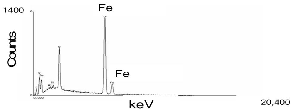
Accelerating voltage 20 KeV, take off angle 35°, live time 93 sec and dead time 13.3 sec showing Si and Fe association.
