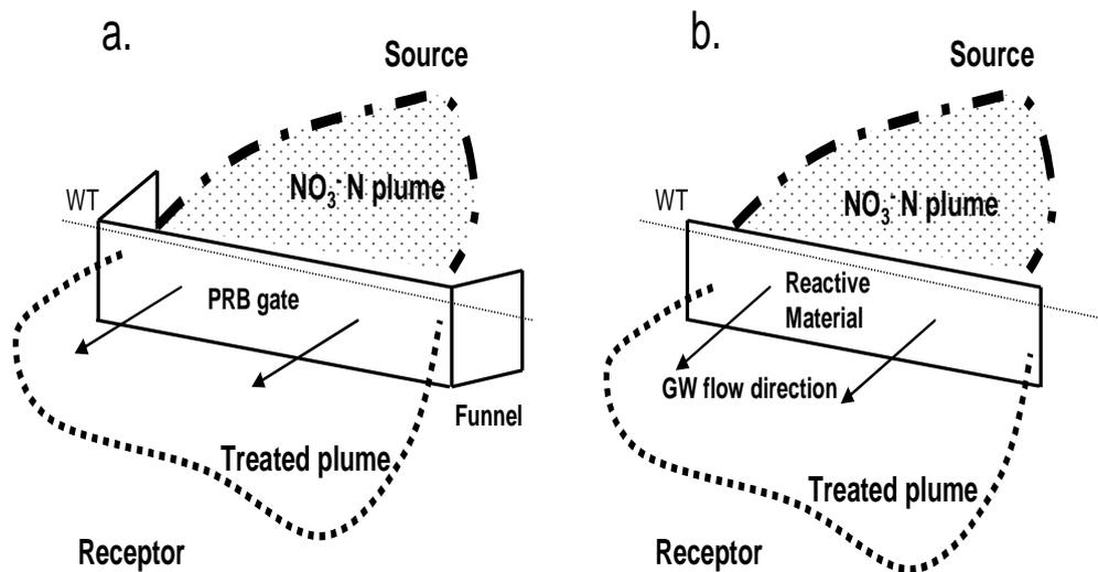
FIGURE 1 A-B FUNNEL AND GATE AND CONTINUOUS TRENCH PRB CONFIGURATIONS.
