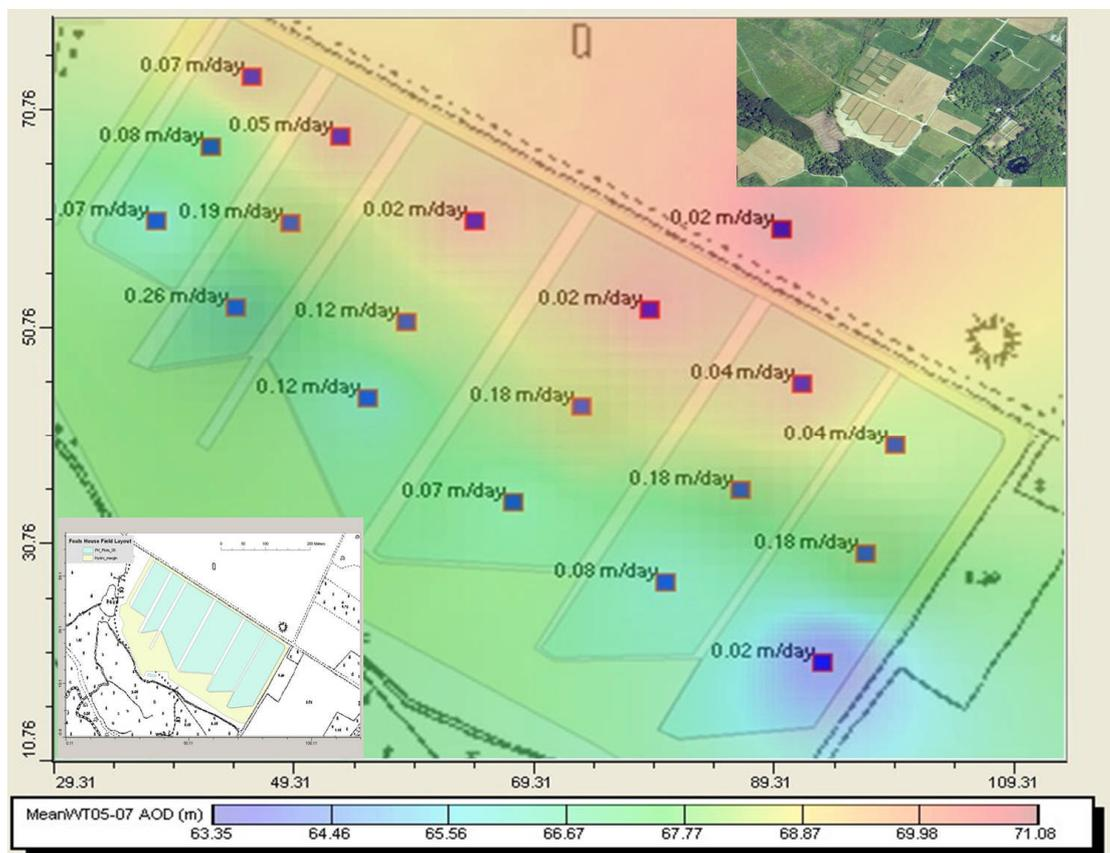
FIGURE 6.1 GROUNDWATER HEADS AND  $K_s$  FOR EACH PIEZOMETER.
