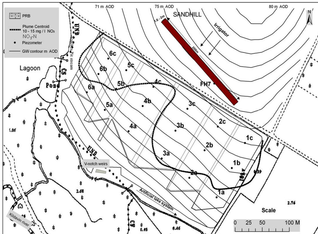
Flow from high to low hydraulic head contours at right angles to contours. Plume centroid location (from 10 to 15 mg  $\text{NO}_3\text{-N L}^{-1}$ ) PRB orientation, location and dimensions.
