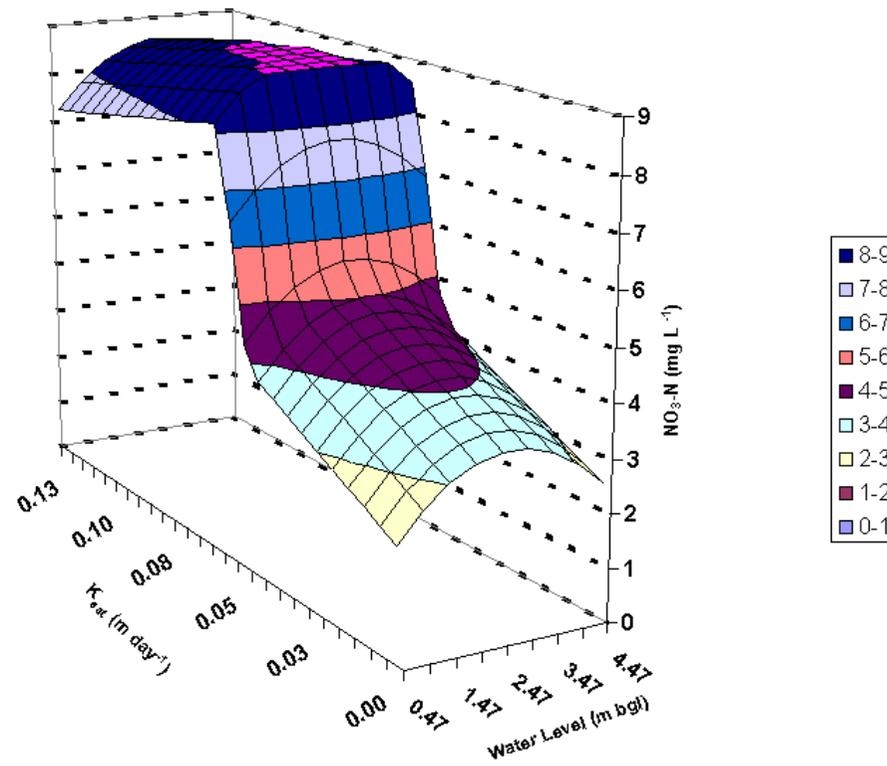
FIGURE 6.8 PREDICTED  $\text{NO}_3\text{-N}$  MODEL USING  $K_s$  AND WATER LEVEL.
