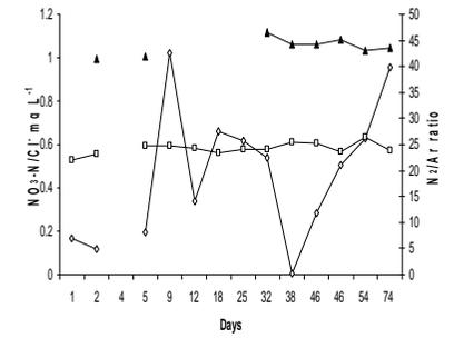
FIGURE 6.6  $N_2/AR$  RATIOS, NITRATE ( $MG L^{-1}$ ) AND CHLORIDE ( $MG L^{-1}$ ) CONCENTRATIONS THROUGHOUT THE EXPERIMENT.
