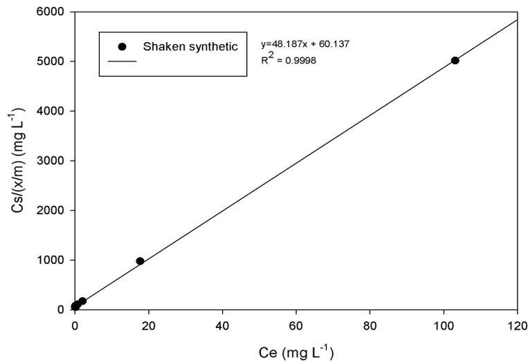
FIGURE 5.2 LANGMUIR ISOTHERM FITTED TO ACTUAL SHAKEN P-AMENDED WATER DATA.
