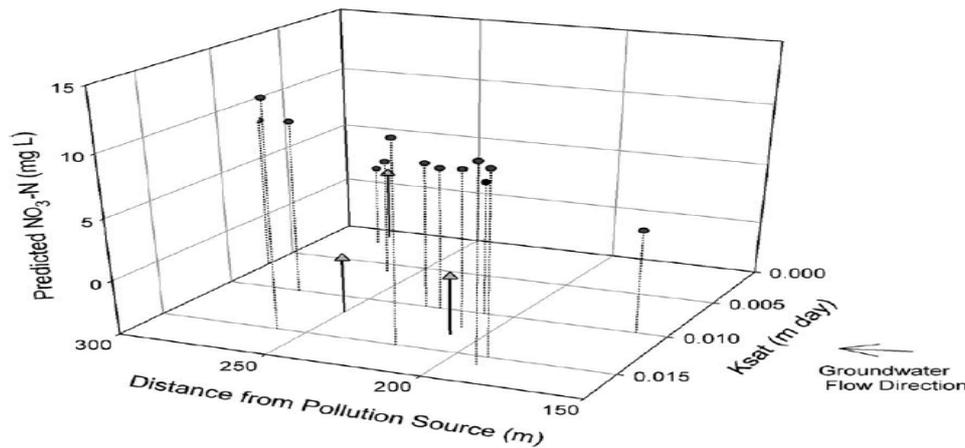
FIGURE 6.4 PREDICTIONS OF MEAN NITRATE FROM FITTED MODEL
