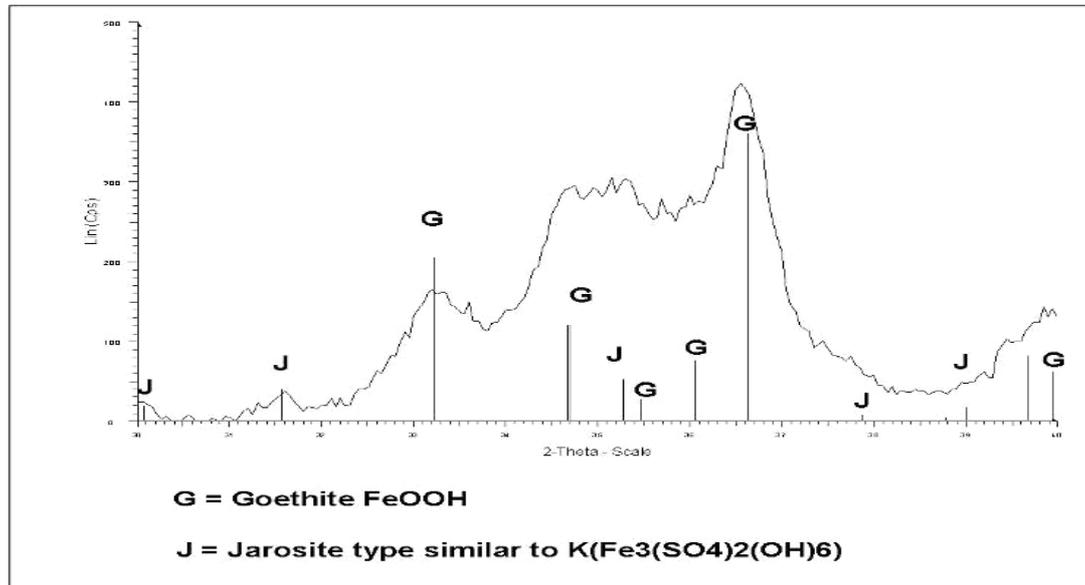
\*Background subtracted file with reference pattern scaled to maximum intensity peaks of Goethite and Jarosite.
