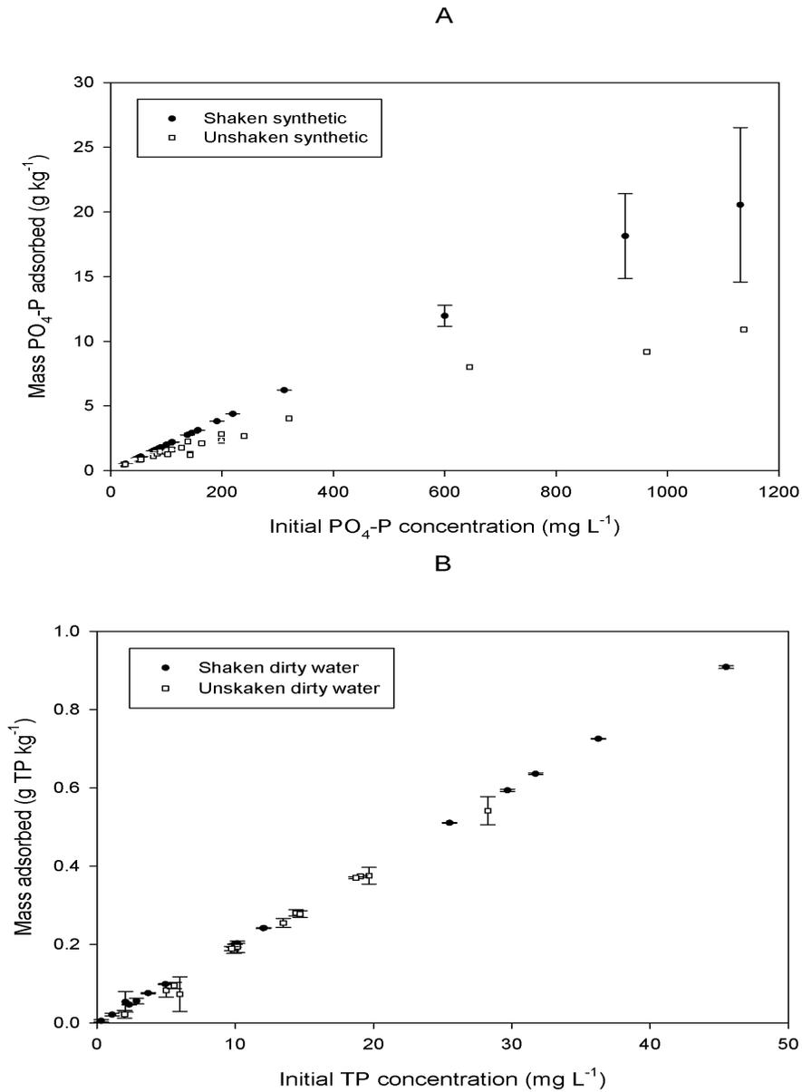
FIGURE 5.1 P REMOVAL IN A) P-AMENDED AND B) DIRTY WATER IN SHAKEN AND UNSHAKEN BATCH EXPERIMENTS
