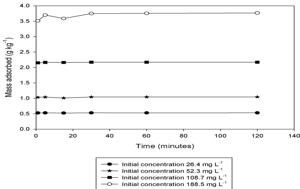
FIGURE 5.3 KINETICS OF P REMOVAL SHOWING 97% REMOVAL OF P WITHIN 5 MIN
