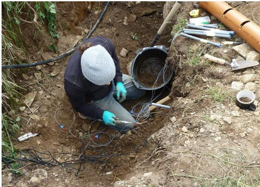
**Fig. 7.5:** Installation of the instruments into the pit-face (grassland, midslope location), using guide holes and soil paste.
