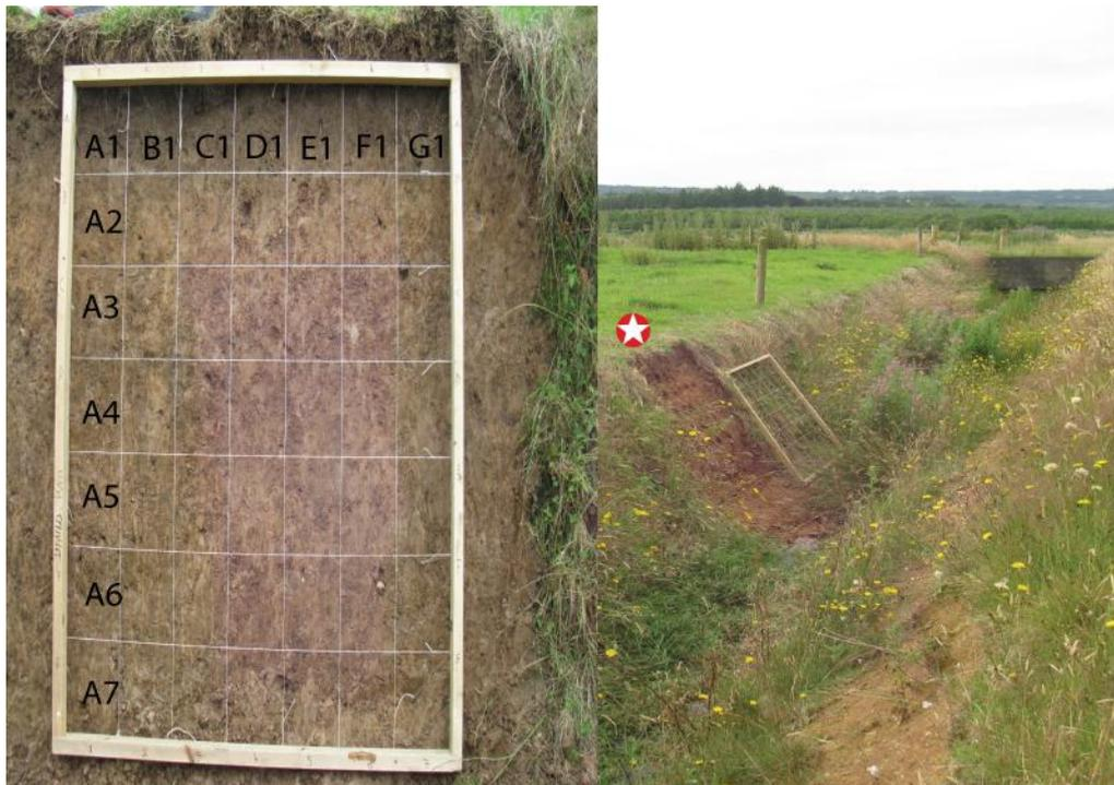
**Fig. 4.1** Soil profile and sample grid location along a deep open drain at a permanent grassland site. C1=Profile A, F1=Profile B.
