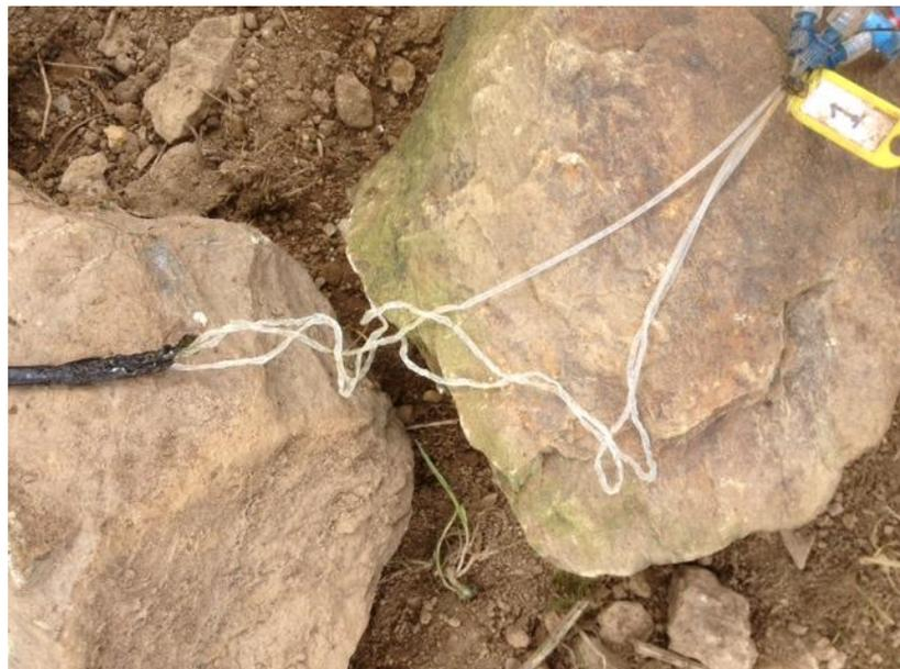
**Fig. 7.10:** Damaged piping for pore water samplers, as a result of vandalism.
