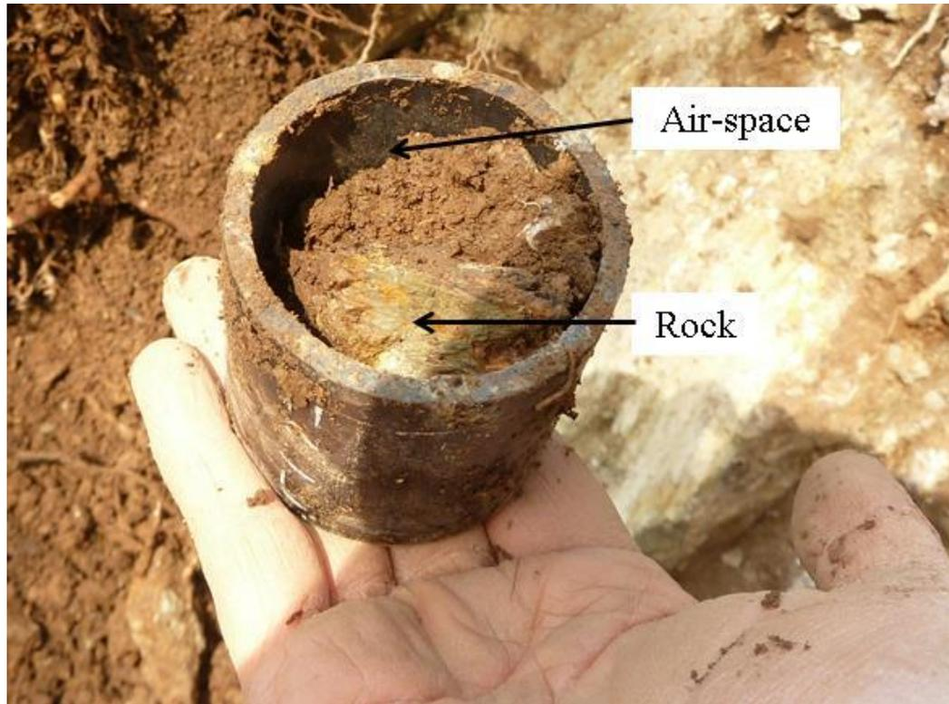
**Fig. 7.20:** An example of a poor soil core, exhibiting both a large stone and an air space. This core is not suitable for SWCC assessment.
