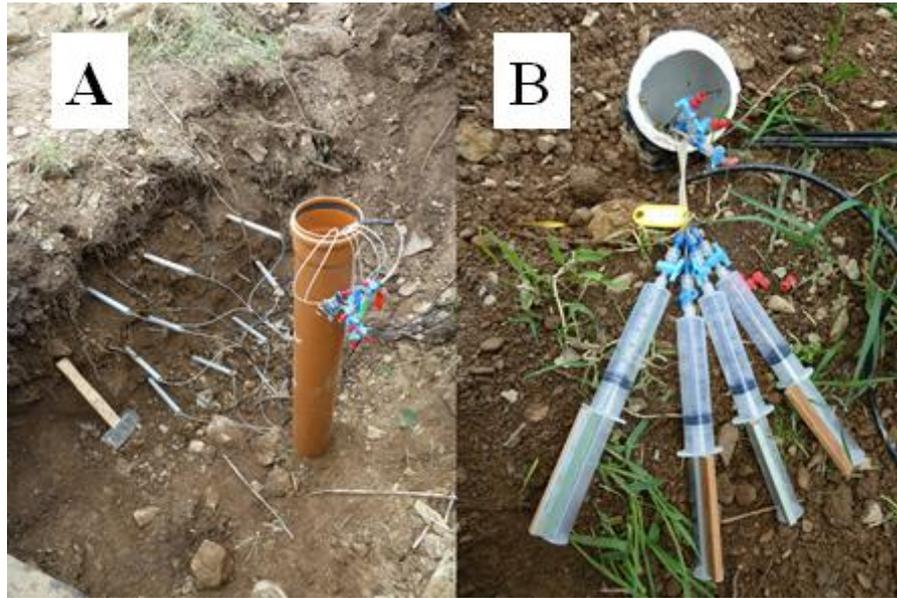
**Fig. 7.6:** (A): Instruments routed from pit-face to surface via piping, prior to backfilling of the excavation. Hammer indicates scale. (B): Lauer-lock syringes collecting pore water at the soil surface, subsequent to backfilling of the excavation. Colour coded tag indicates the depth of the pore water samplers. Both photographs obtained at the grassland, lowslope location.
