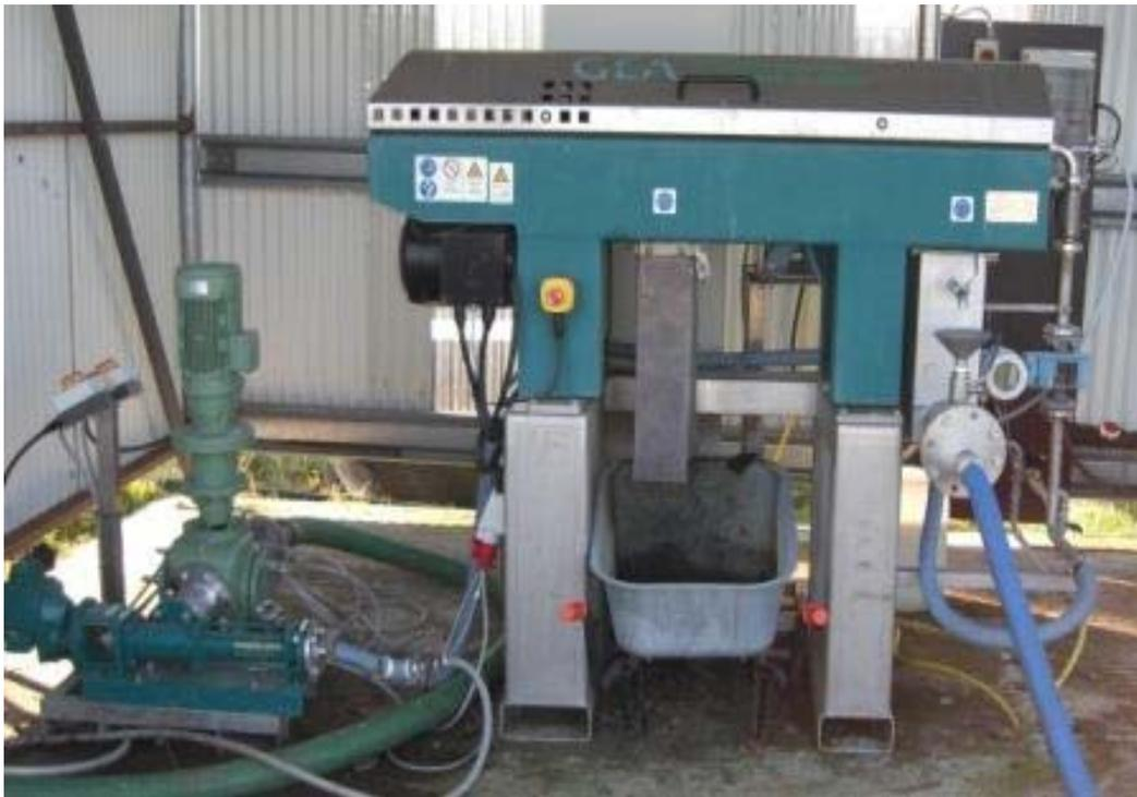
**Figure 3.1** Decanter centrifuge used for the separation of pig manure into a solid and liquid fraction
