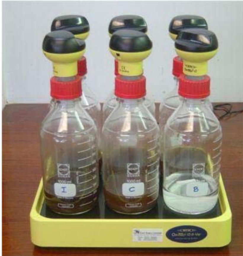
**Figure 3.3** Oxitop Control System used for measuring the Oxygen Uptake Rate
