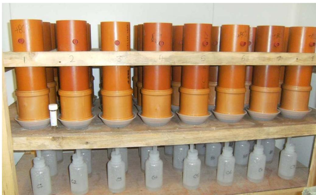
**Figure 7.2** PVC columns used to contain soil for the leaching experiment
