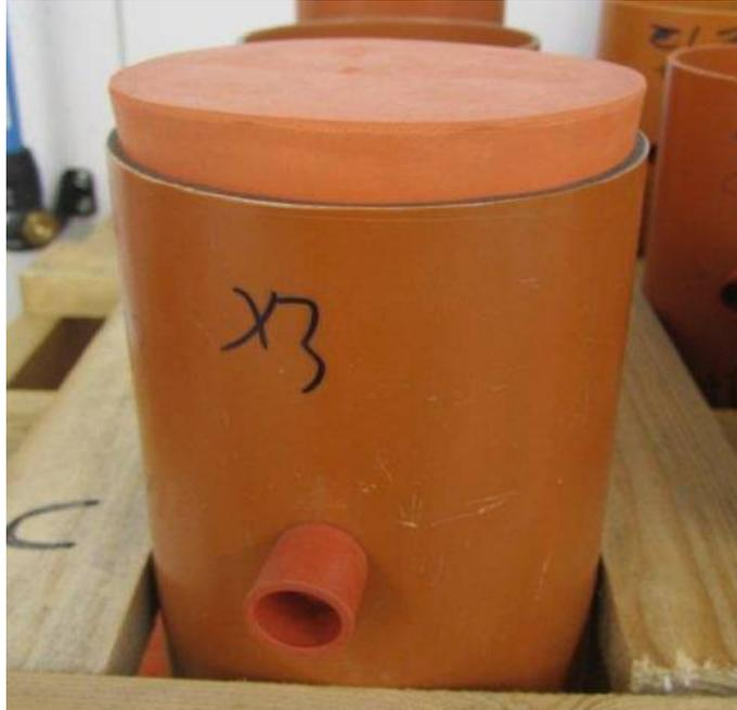
**Figure 8.1** The rubber stopper used to seal the column headspace and the septum through which a gas sample was taken.
