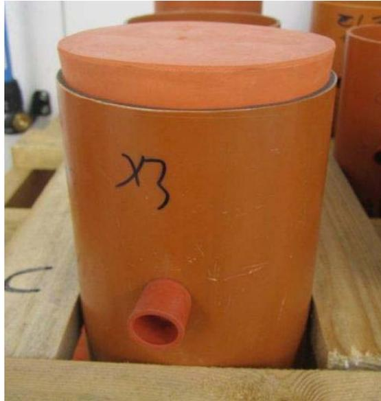
**Figure 5.1** PVC column with rubber stopper.
