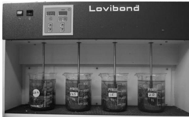
Figure 1. The agitator experimental setup.
