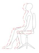
Seat Slide Adjustment -Front Left Hand Paddel - Lift Paddle to slide seat forward, release to lock, lift again to return seat.
