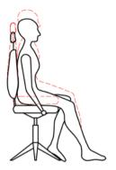
Seat Height Adjustment -Right Hand Paddle - Lift paddle up whilst off seat to raise seat height, lift paddle whilst seated to lower seat height.
