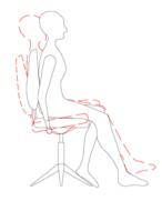
Synchro Seat and Back Angle Adjustment - Rear Right Hand Paddle -Lift paddle up to release and down to lock, Lockable in four positions, with underseat tension
