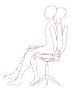
Synchro Seat and Back Angle Adjustment -Left Hand Lever. Press down to release and Up to lock the tilt position. Tension is controled under
