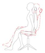
Synchro Seat and Back Angle Adjustment -Left Hand Lever. Press down to release and Up to lock the tilt position. Tension is controlled under the seat.
