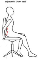
Pump out Lumbar Support -Located beow the backrest to the right. Squeeze the hand pump with right hand. To release the pressure press the button on the hand pump.
