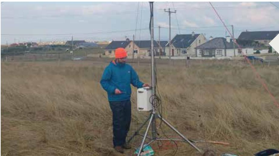
Geography PhD student Guillermo Castro Camba is pictured setting up a portable Automatic Weather Station on the sand dunes in Magharees (An Machaire), Co. Kerry. He is using the low-power device to collect high frequency meteorological measurements in order to examine how the weather impacts our coastline. The research is part of an OPW-funded project by Dr Eugene Farrell and Dr Kevin Lynch (Geography) that examines **long-term beach-dune response and recovery to storms**.
