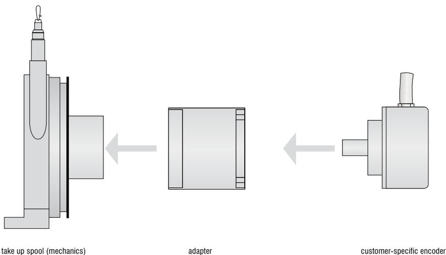
For the customer-specific encoder or potentiometer various draw-wire mechanics are available with measuring ranges up to 50m.
