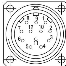
Pin 2 and Pin 12 are internally connected as well as Pin 11 and 10. For cable length > 10m twisted pair wires are required.
