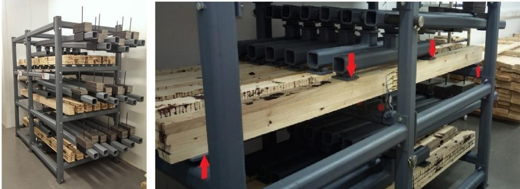
**Fig. 4.** Creep test frame: (a) Loaded creep test frame in a constant climate condition at a temperature of  $20 \pm 2$  °C and at a relative humidity of  $65 \pm 5$ %, (b) Creep test beam loaded in four-point bending.
