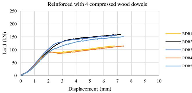
Figure 7.3 Load-deformation for specimens with 4 dowels
