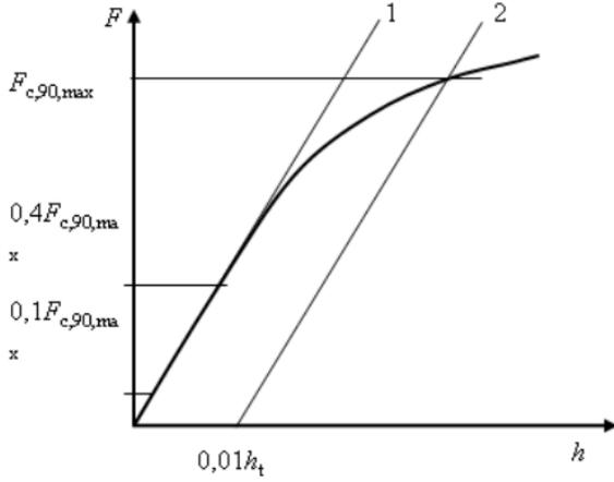
Figure 2.1 Load-deformation curve [7]
