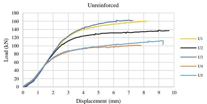
Figure 7.1 Unreinforced specimens load-deformation curves
