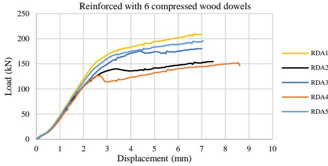
Figure 7.2 Load-deformation for specimens with 6 dowels
