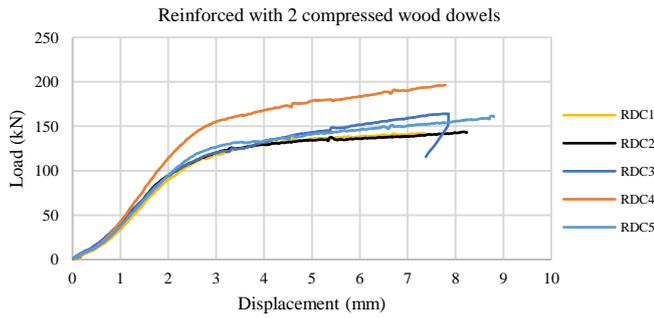
Figure 7.4 Load-deformation for specimens with 2 dowels
