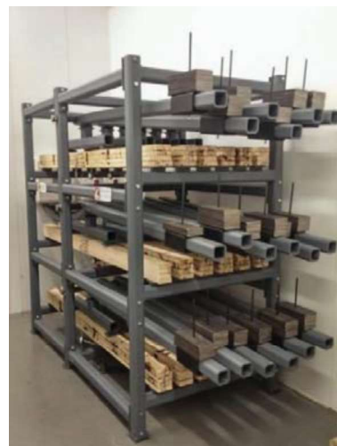
Figure 5. Loaded Creep Frame in Constant Climate
