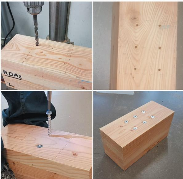
**Figure 3.** Preparation of self-tapping screw reinforced specimen.
