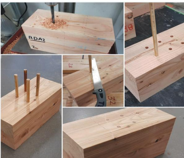
**Figure 4.** Preparation of densified wood reinforced specimen.
