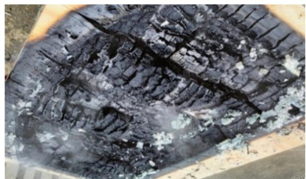
**Figure 10.** W-1 panel after the fire test showing pieces of localized char fall-off.
