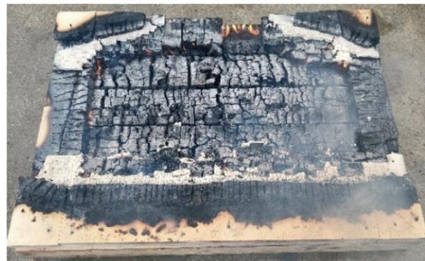
Figure 18. A photo was taken after the test showing the fall-off of cladding and outer layer of CLT panel: W-12.5FP25PW.
