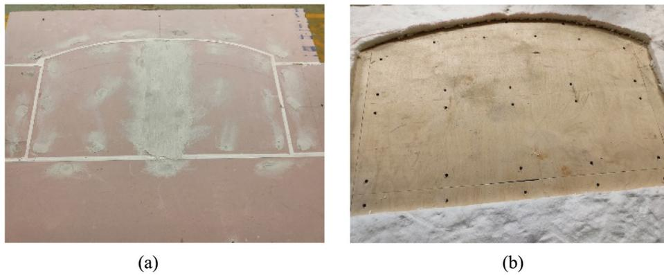
**Figure 5.** W-12.5FP25PW, (a) 12.5 mm Fireline gypsum plasterboard with joints placed between the CLT panel and the outer plywood layer, (b) Exposed 25 mm plywood layer with joints.
