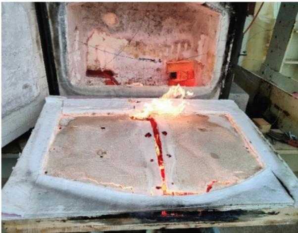
**Figure 22.** Fireline gypsum plasterboard remaining in place for the duration of the test W-15FPJ.
