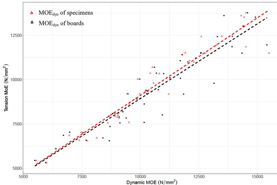
**Figure 3**—Relationship between MoE<sub>dyn</sub> of the test specimen and the board with the MoE<sub>t</sub>.
