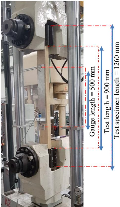
Figure 1—Set up of tension test.
