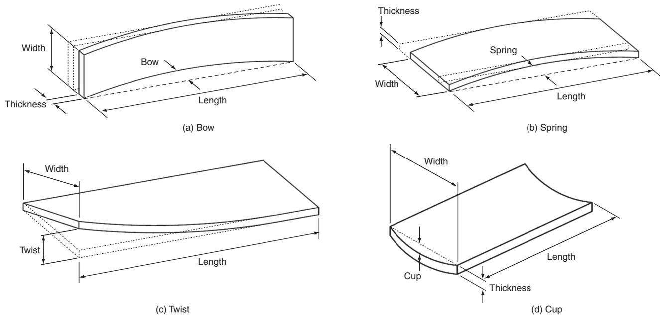
Figure 4 Geometrical imperfections and distortion in timber
