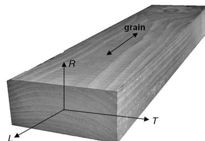
Figure 3 Orthotropic directions for wood properties
