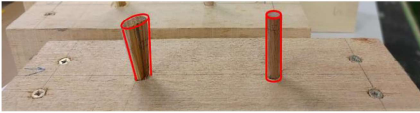
Figure 7: Shape of the dowels of Series C after the treatment.
