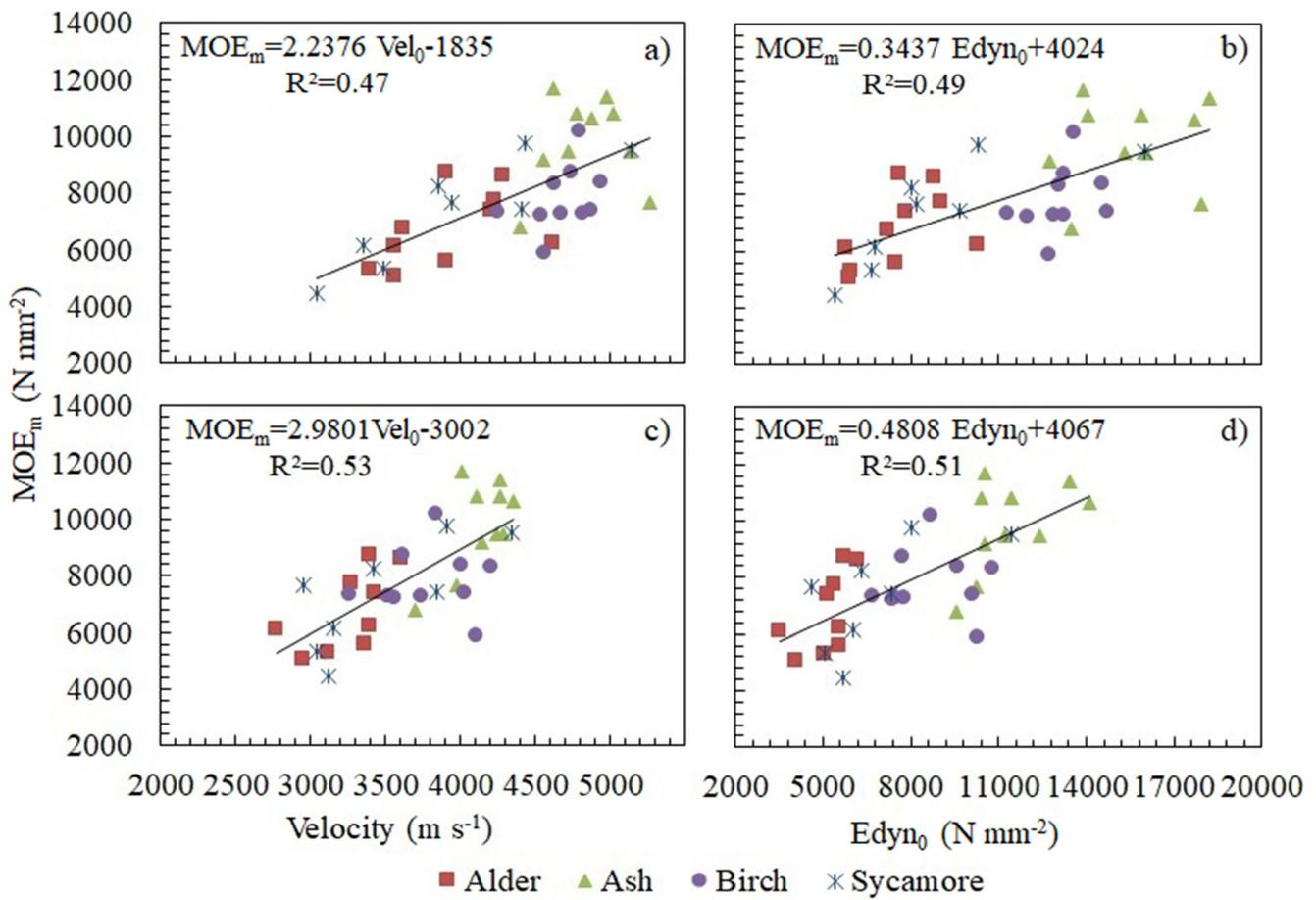
**Fig. 4** Linear regressions between static  $MOE_m$  and (a) TreeSonic velocity, (b) TreeSonic  $Edyn_0$ , (c) MTG velocity, and (d) MTG  $Edyn_0$
