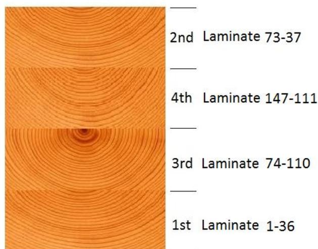
Figure 2. Glulam beam lay up.
