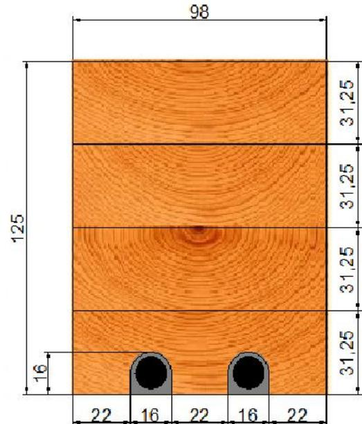
Figure 4. Reinforcement detail.
