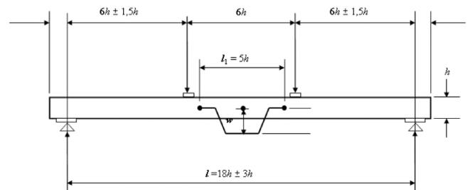
Figure 5. Beam bending set-up [18].
