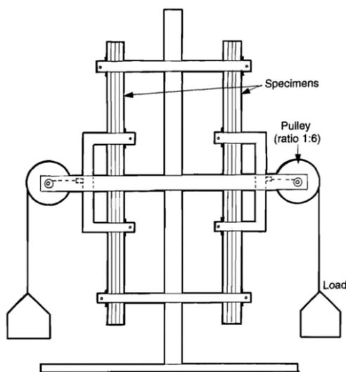
Figure 1. Vertical creep experimental rig [14].
