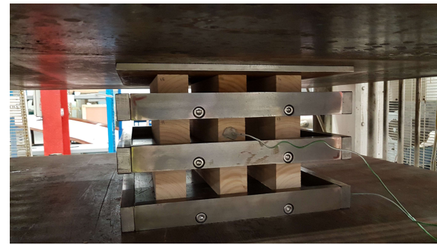
Figure 2: Compressed wood press apparatus a) Press elevation showing different layer dimensions and associated compression ratios - Timber is in yellow, final densified wood is in red (dimensions in mm), b) press apparatus with timber specimens between the heated platens of the press.
