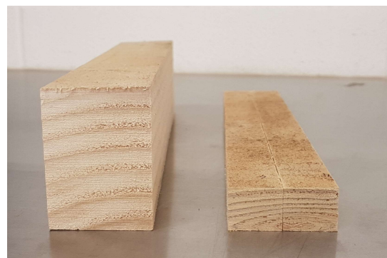
Figure 1: Un-compressed Sitka spruce compared to a similar specimen that has been subjected to thermo-mechanical compression to form Compressed Sitka spruce
