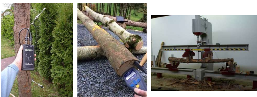
Fig. 2 : NDT measurements on standing trees(a), logs (b) and mechanical test (c)
