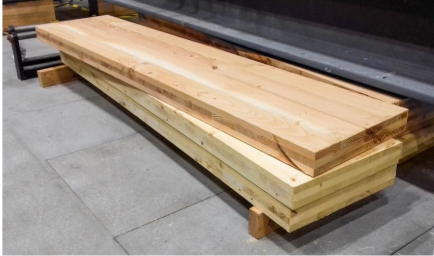
Figure 2. CLT panels from recovered timber in the NUIG laboratory
