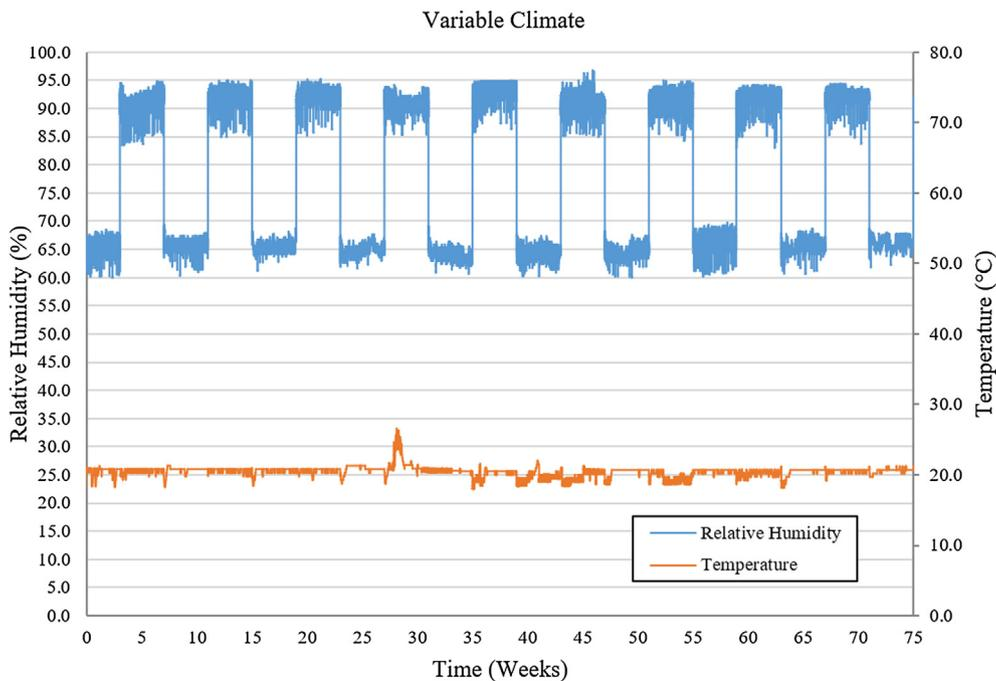
Fig. 3. Relative humidity and temperature data recorded in the variable climate chamber.
