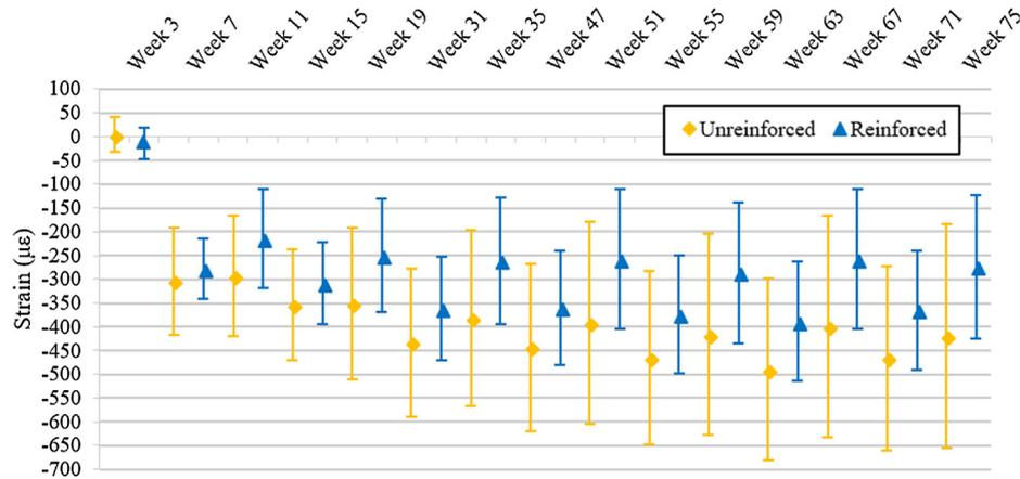
Fig. 16. Mean mechano-sorptive strain ( $\epsilon_{ms}$ ) and associated standard deviations on the compression face of unreinforced and reinforced beams.
