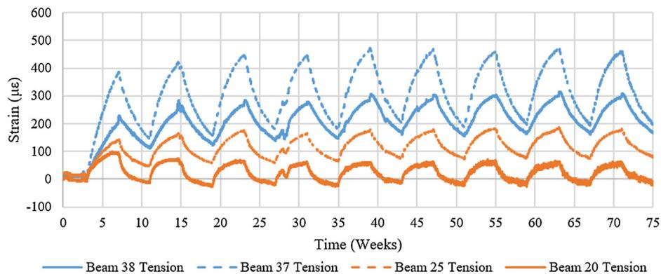
Fig. 14. Swelling/shrinkage strain results ( $\epsilon_s$ ) on the tension face of unreinforced and reinforced beams.
