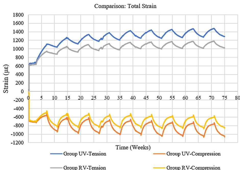
Fig. 8. Mean total longitudinal strain on the tension and compression faces of Group UV and Group RV ( $\epsilon_T = \epsilon_e + \epsilon_{ve} + \epsilon_{ms} + \epsilon_s$ ).
