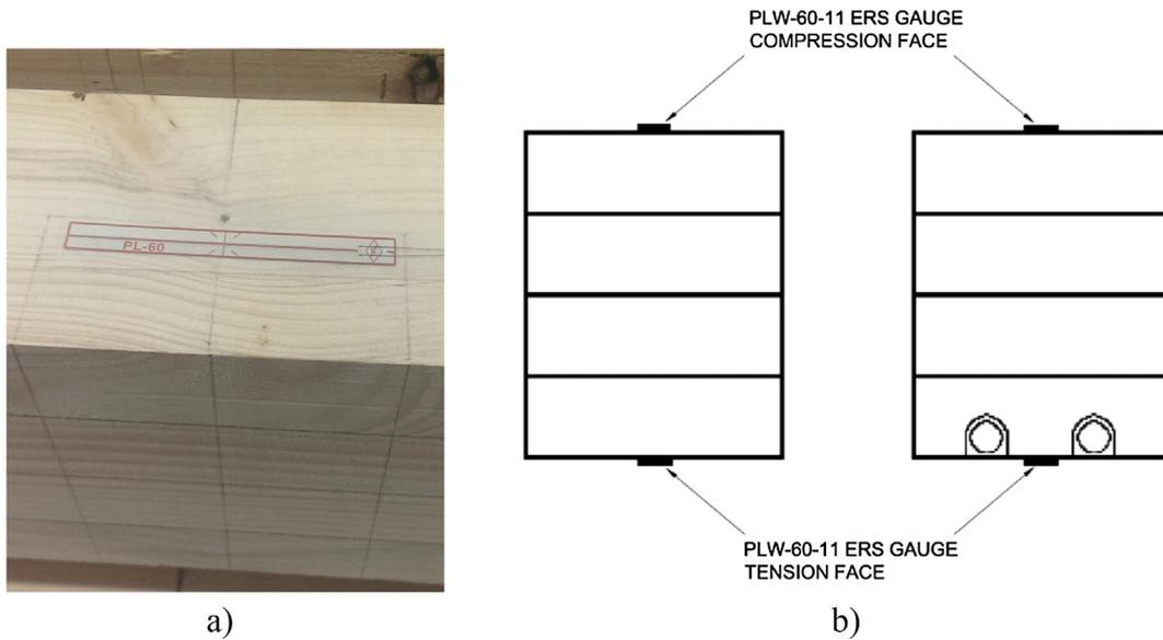
Fig. 2. PLW-60-11 ERS gauge, (a) PLW-60-11 ERS gauge alignment, (b) PLW-60-11 ERS gauge positions on the tension and compression face of the unreinforced and reinforced beams.
