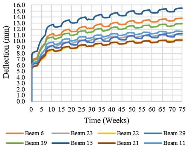
Fig. 4. Group UV mid-span deflection (mm) results.
