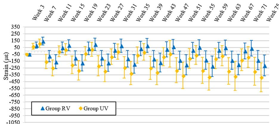
Fig. 11. Mean and standard deviation of total longitudinal creep strain on the compression face.
