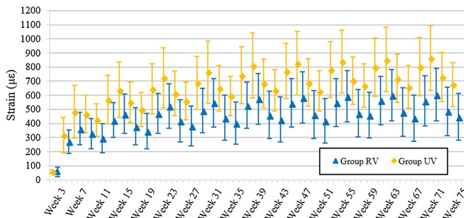
Fig. 10. Mean and standard deviation of total longitudinal creep strain on the tension face ( $\epsilon_{creep} = \epsilon_{ve} + \epsilon_{ms} + \epsilon_s$ ).
