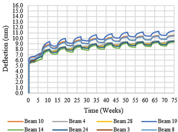
Fig. 5. Group RV mid-span deflection (mm) results.
