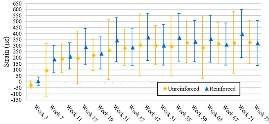
Fig. 15. Mean mechano-sorptive strain ( $\epsilon_{ms}$ ) and associated standard deviations on the tension face of unreinforced and reinforced beams.
