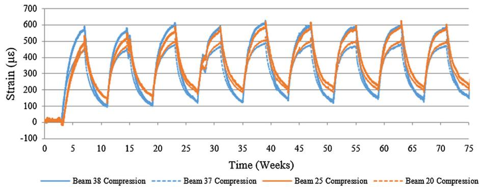
Fig. 13. Swelling/shrinkage strain results ( $\epsilon_s$ ) on the compression face of unreinforced and reinforced beams.
