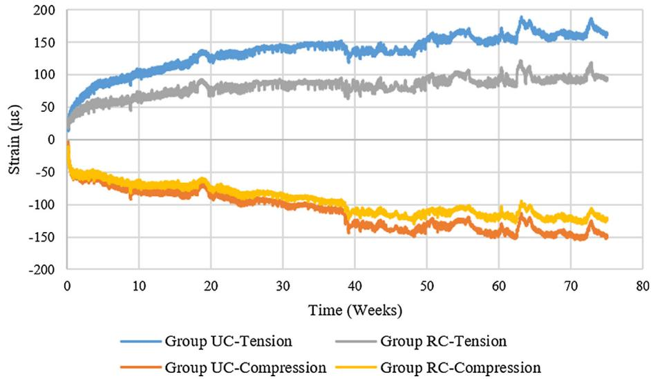
Fig. 12. Mean longitudinal viscoelastic creep strain ( $\epsilon_{ve}$ ) on the tension and compression faces of Group UC and Group RC.
