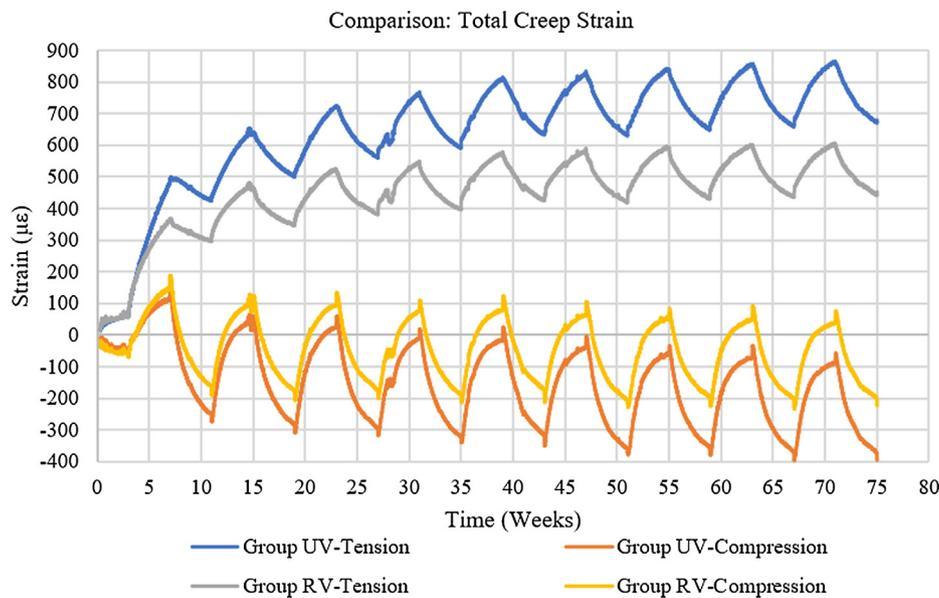
Fig. 9. Mean longitudinal creep strain on the tension and compression faces of Group UV and Group RV ( $\epsilon_{creep} = \epsilon_{ve} + \epsilon_{ms} + \epsilon_s$ ).
