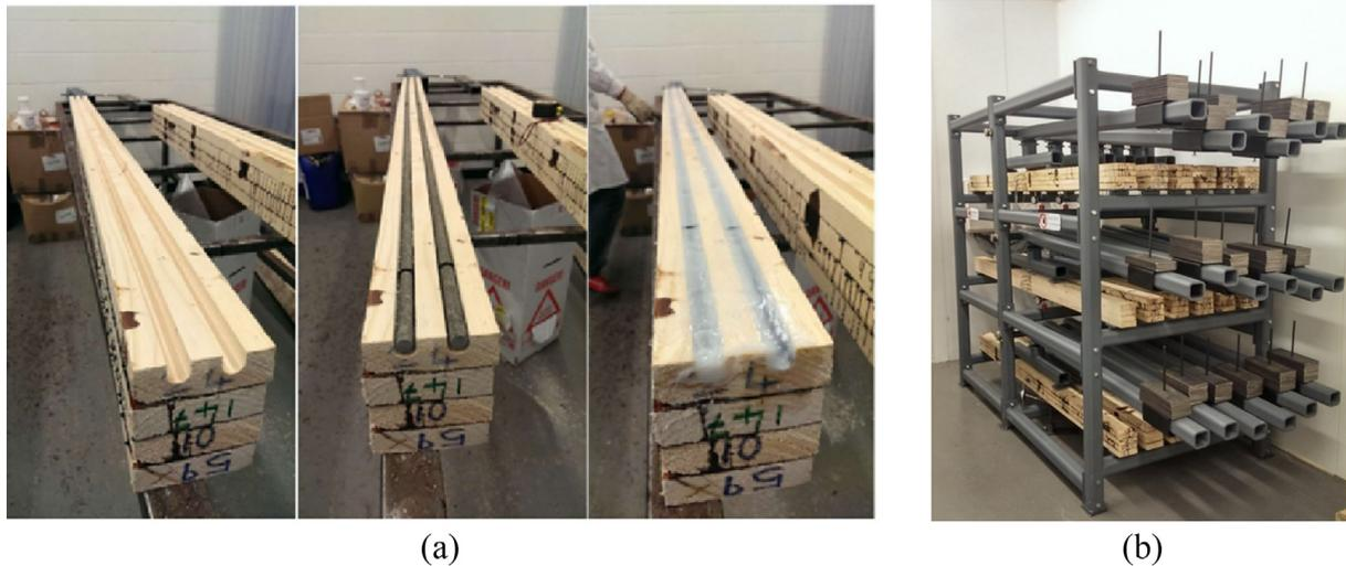
Fig. 1. Reinforced beams: (a) Manufacture of reinforced members, (b) 18 beams loaded in the creep test frame.
