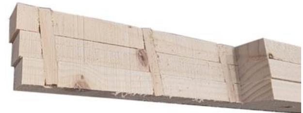
**Figure 6:** Interlaminar slip, stepped profile and dowel-timber embedment.
