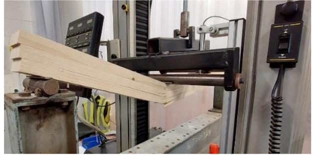
**Figure 5:** Failure behaviour of DLT member (DLT - 2)
