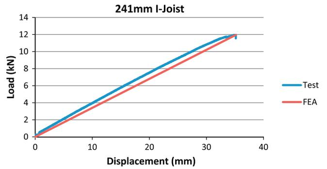
Fig. 8. Test versus FE Load-deflection results for I-joist 241\_3.
