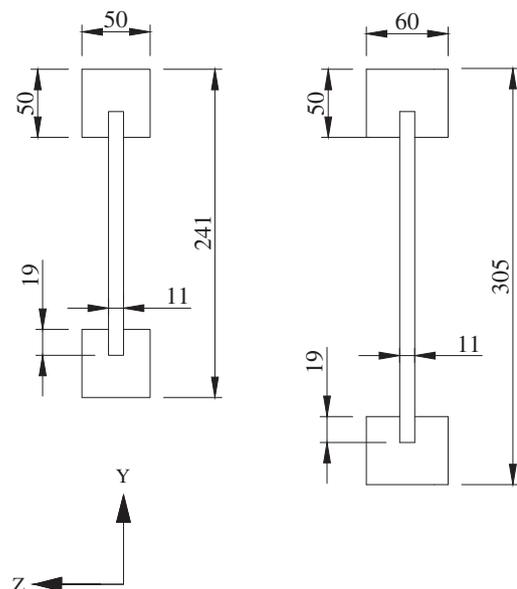
Fig. 2. Section through joists. Dimensions in mm.
