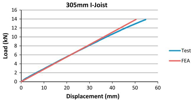
Fig. 9. Test versus FE Load–deflection results for I-joist 305\_4.
