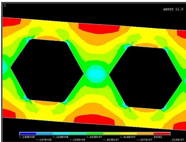
Fig. 12. Web shear stress distribution ( $\text{Nm}^{-2}$ ) at peak load between 3rd and 4th hole of 241 mm I-joist.
