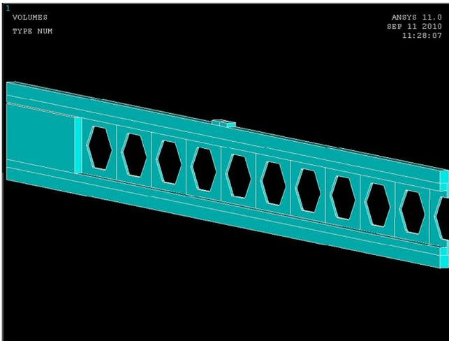
Fig. 3. Geometric quarter FE model used for 4 point bend test.
