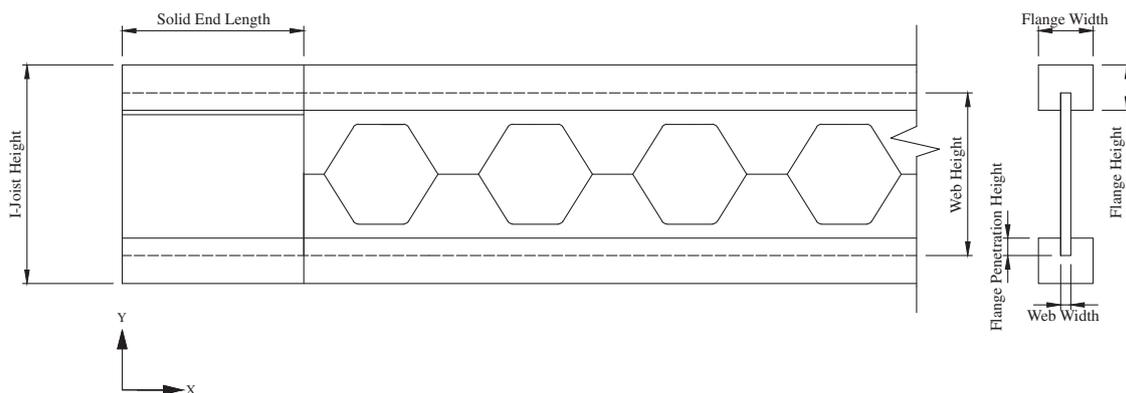
Fig. 5. Longitudinal section and cross section of castellated I-joist with geometric parameters.
