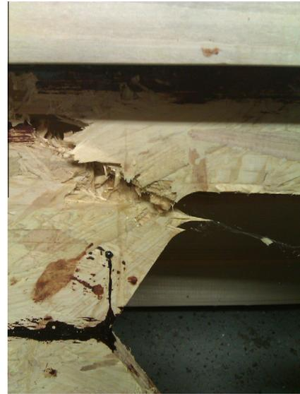
Fig. 10. Tension failure at corner of opening.
