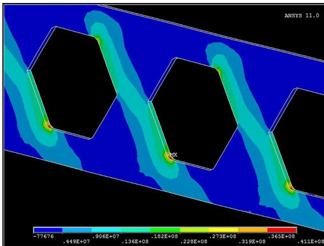
Fig. 11. First principal stress distribution in web ( $\text{Nm}^{-2}$ ).
