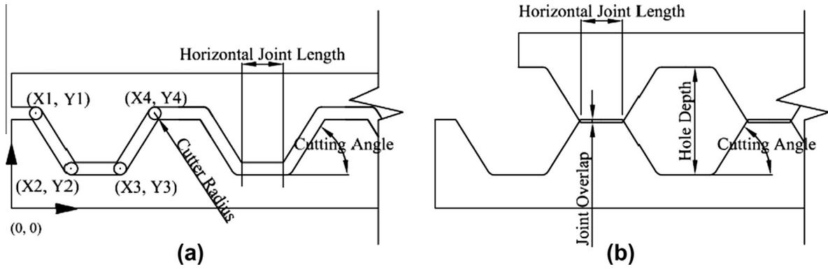
Fig. 6. Web geometric parameters (a) OSB blank with cutting profile and (b) resulting castellated web.
