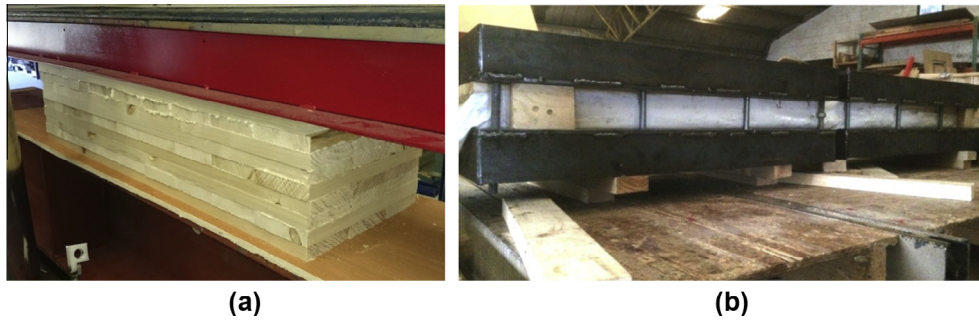
Fig. 1. Manufacture of CLT panel using (a) hydraulic press, (b) bolts and steel plates.
