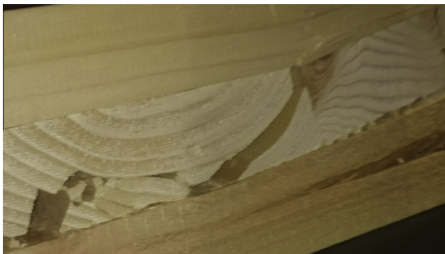
Fig. 8. Rolling shear failure in Specimen S-3-40-2.
