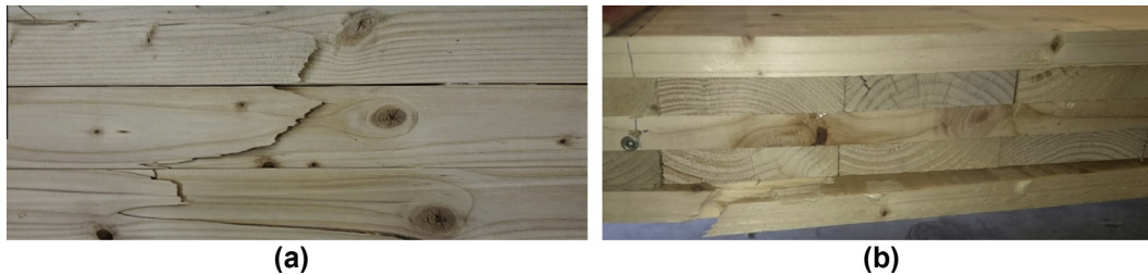
Fig. 3. (a) Tensile failure on bottom of Specimen B-3-20-1; (b) tensile failure followed by delamination of Specimen B-5-20-1.
