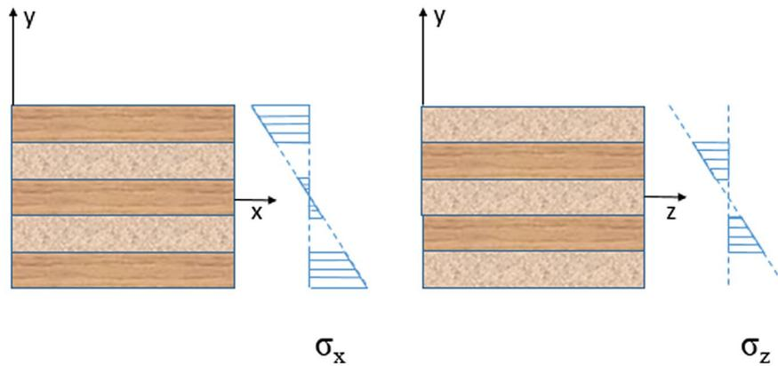
Figure 4. Stress distribution in CLT:  $\sigma_x$  major axis bending;  $\sigma_y$  minor axis bending.
