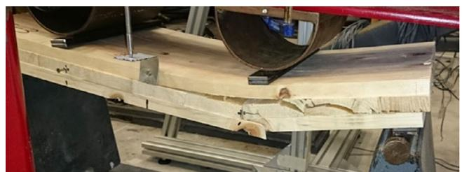
Figure 18. Rolling shear failure of Irish CLT panel.
