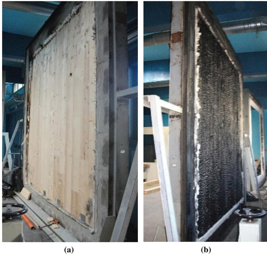
Figure 6. CLT panel after 1 h fire test (a) unexposed face; (b) exposed face.
