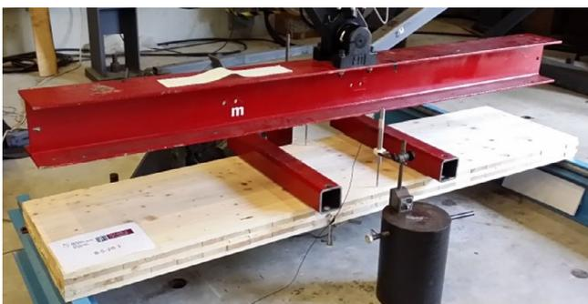
Figure 17. Out-of-plane bending test on Irish CLT panel.
